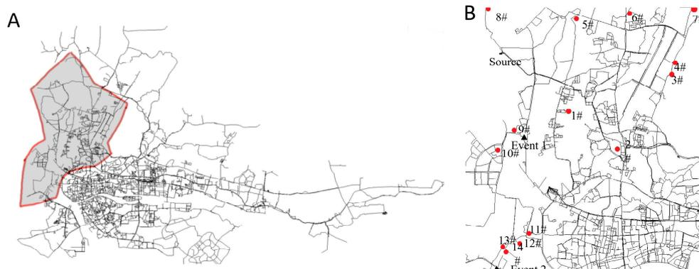
**Figure 3.** Water distribution system (WDS) in Guangzhou: (A) the area supplied by the Shimen water plant and (B) the 14 sensor locations; the black triangles identify the locations of observed burst events.
