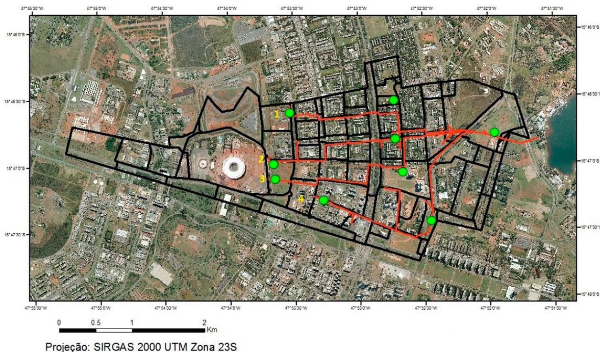
**Figure 6.** Urban Drainage Design with position and location of detention ponds in the galleries numbered 1 to 4.
