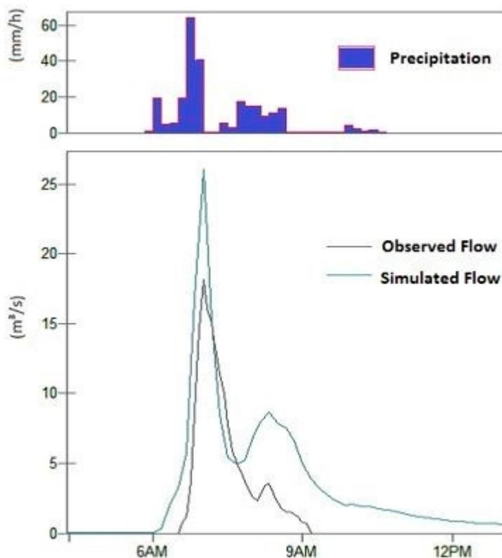
**Figure 8.** Hydrograms between the model simulated and observed data.
