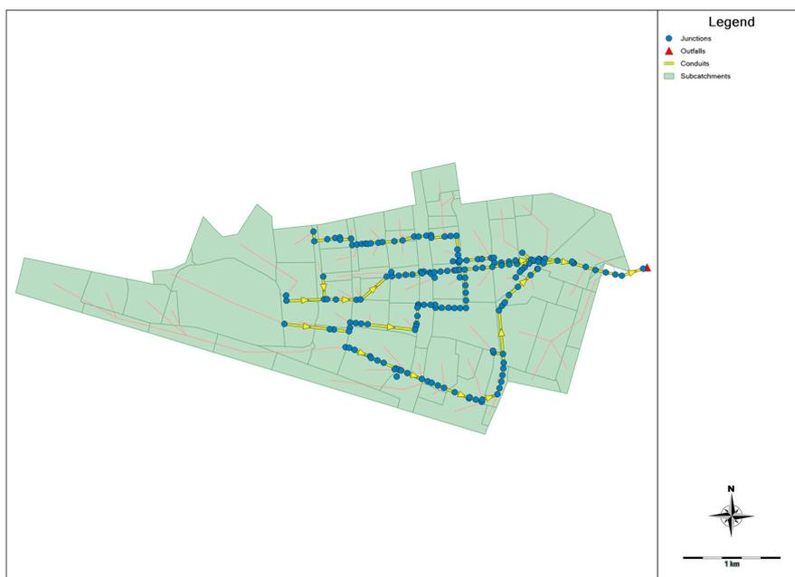
**Figure 3.** Drainage System in the Iate Basin, with junction, conduits, outfalls, and sub-basins at PCSWMM program.
