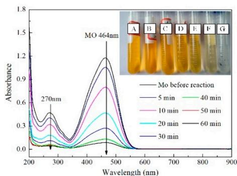
**Figure 5.** UV-vis patterns of degradation of MO.
