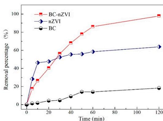
**Figure 4.** Comparative degradation of MO using different materials. The dosage of BC, nZVI, and BC-nZVI were 3 g/L, 0.5 g/L, and 0.5 g/L (the dry weight of nZVI in BC-nZVI used) with an initial MO concentration of 200 mg/L, temperature of 25 °C, and original pH.
