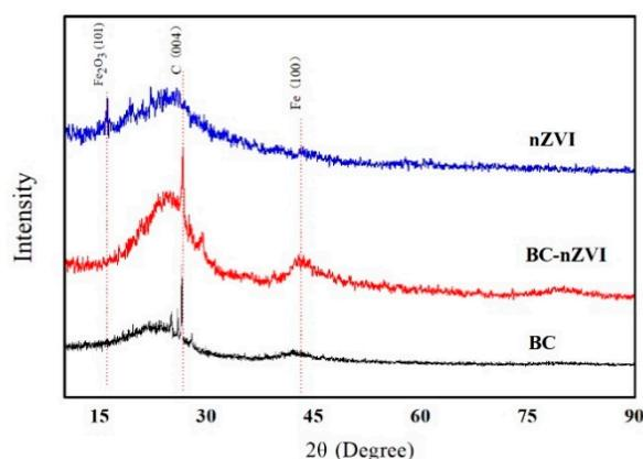
Figure 3. XRD pattern of nZVI, BC, and BC-nZVI.
