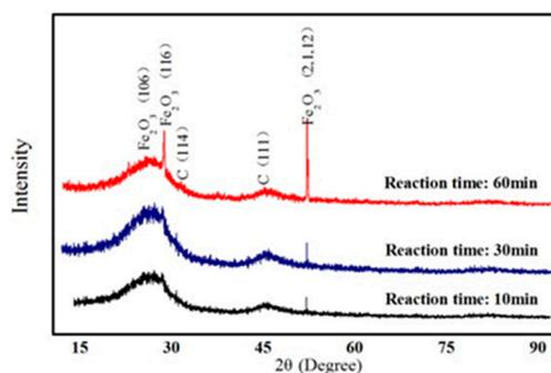
Figure 6. XRD pattern of BC-nZVI after reaction.
