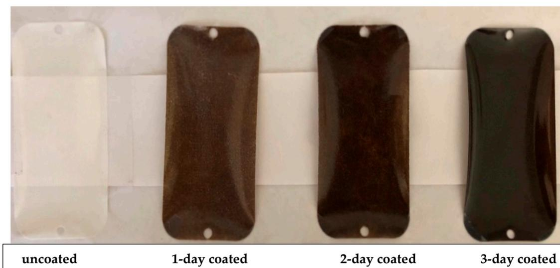
Figure 5. The changes in the colors of the membranes due to coating.
