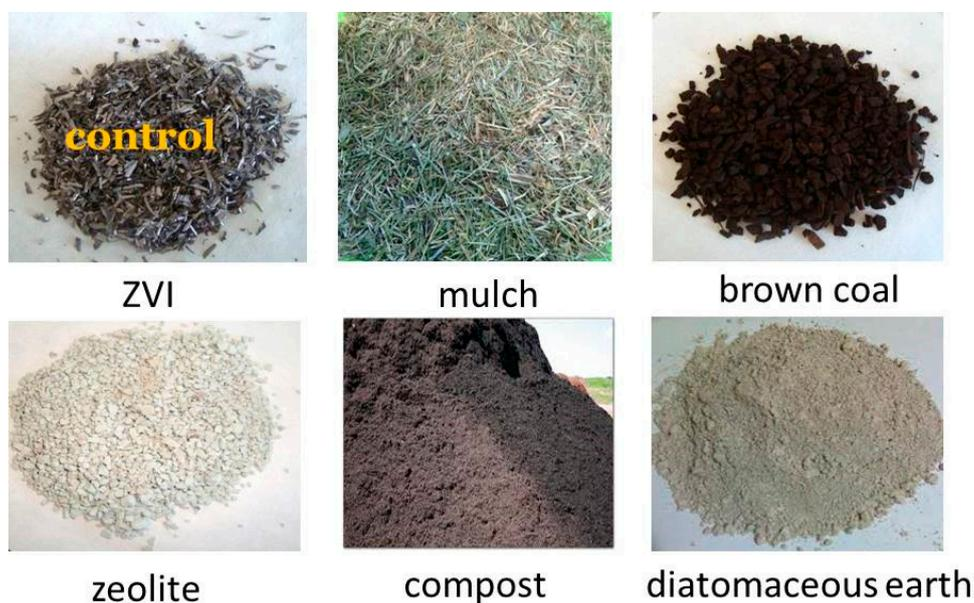
Figure 1. Reactive materials tested.
