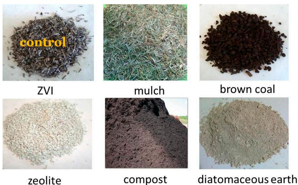
Figure 1. Reactive materials tested.
