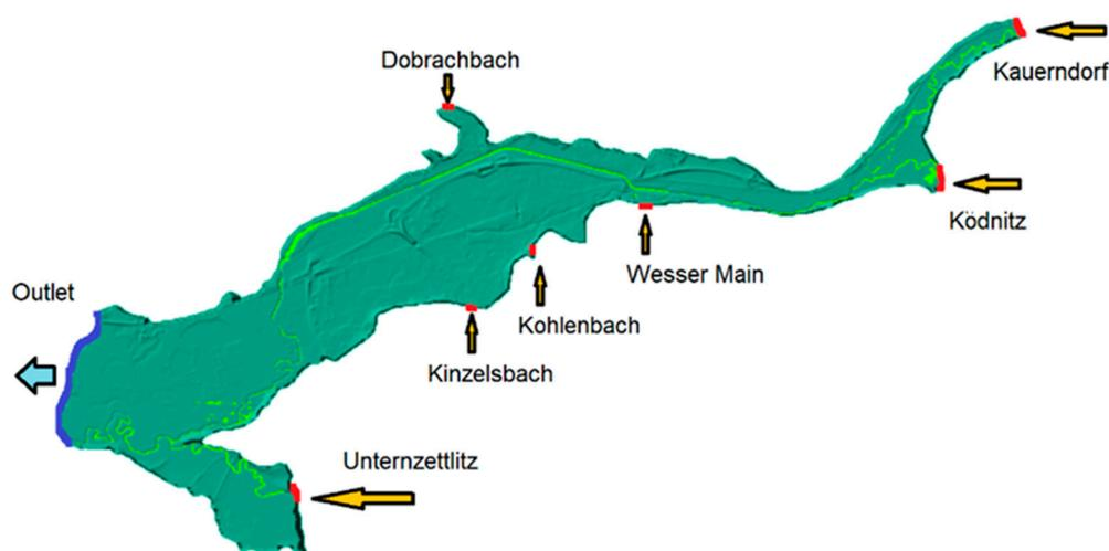
Figure 2. Model grid area with marked Inflows (red) and outflows (blue) boundary conditions.
