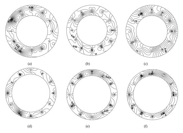
**Figure 17.** Radial flow velocity distribution of annular gap sections of the capsules: (a) L/d = 2.5, rear section; (b) L/d = 2.5, middle section; (c) L/d = 2.5, front section; (d) L/d = 2.14, rear section; (e) L/d = 2.14, middle section; and (f) L/d = 2.14, front section.
