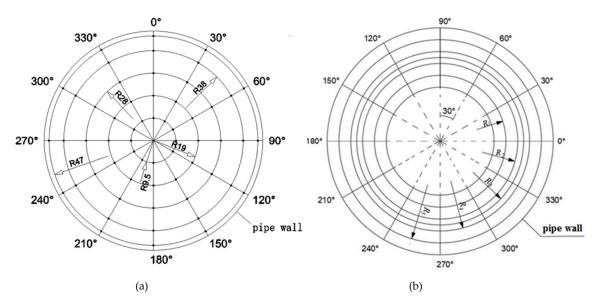
**Figure 3.** Layout of measuring points of sections: (**a**) the front and rear sections of capsule and (**b**) the annular gap section.
