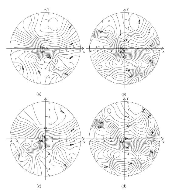
**Figure 6.** Circumferential velocity distributions of the upstream sections of capsules: (a) L/d = 2.5, Z = 3 m; (b) L/d = 2.14, Z = 3 m; (c) L/d = 2.5, Z = 0.1 m; and (d) L/d = 2.14, Z = 0.1 m.
