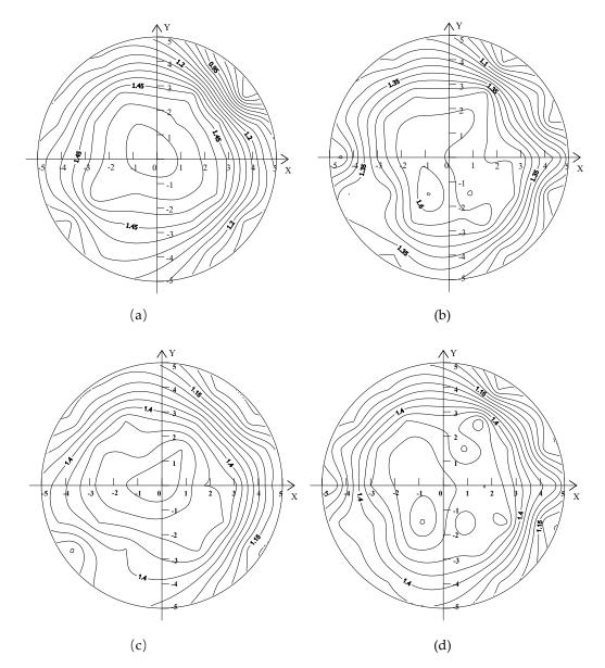
**Figure 5.** Axial velocity distributions of the upstream sections of capsules: (a) L/d = 2.5, Z = 3 m; (b) L/d = 2.14, Z = 3 m; (c) L/d = 2.5, Z = 0.1 m; and (d) L/d = 2.14, Z = 0.1 m.
