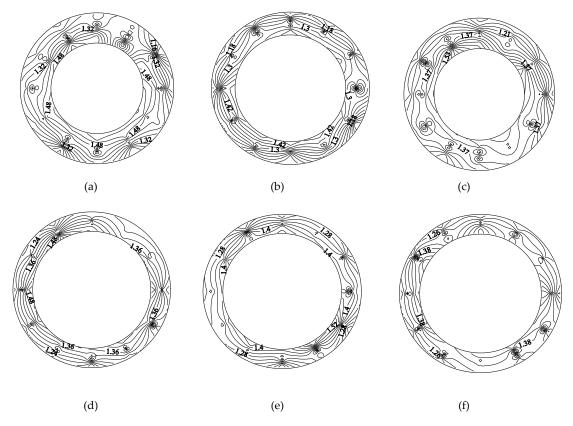
**Figure 11.** Axial flow velocity distribution of annular gap sections of the capsules: (a) L/d = 2.5, rear section; (b) L/d = 2.5, middle section; (c) L/d = 2.5, front section; (d) L/d = 2.14, rear section; (e) L/d = 2.14, middle section; and (f) L/d = 2.14, front section.
