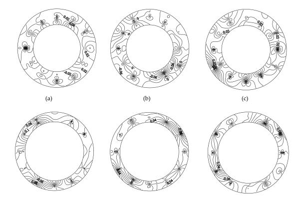
**Figure 14.** Circumferential flow velocity distribution of annular gap sections of the capsules: (a) L/d = 2.5, rear section; (b) L/d = 2.5, middle section; (c) L/d = 2.5, front section; (d) L/d = 2.14, rear section; (e) L/d = 2.14, middle section; and (f) L/d = 2.14, front section.
