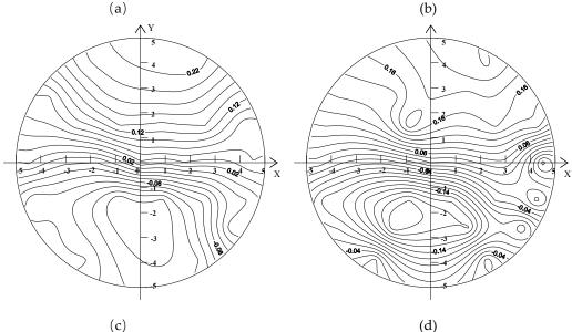
**Figure 9.** Circumferential velocity distribution of the downstream sections of capsules: (a) L/d = 2.5, Z = 0.2 m; (b) L/d = 2.14, Z = 0.2 m; (c) L/d = 2.5, Z = 3 m; and (d) L/d = 2.14, Z = 3 m.
