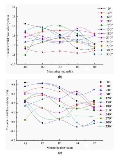
**Figure 15.** Circumferential velocity of the same polar axis: (**a**) rear section; (**b**) middle section; and (**c**) front section.
