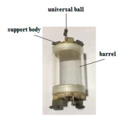
Figure 1. Structural diagram of wheeled capsule.
