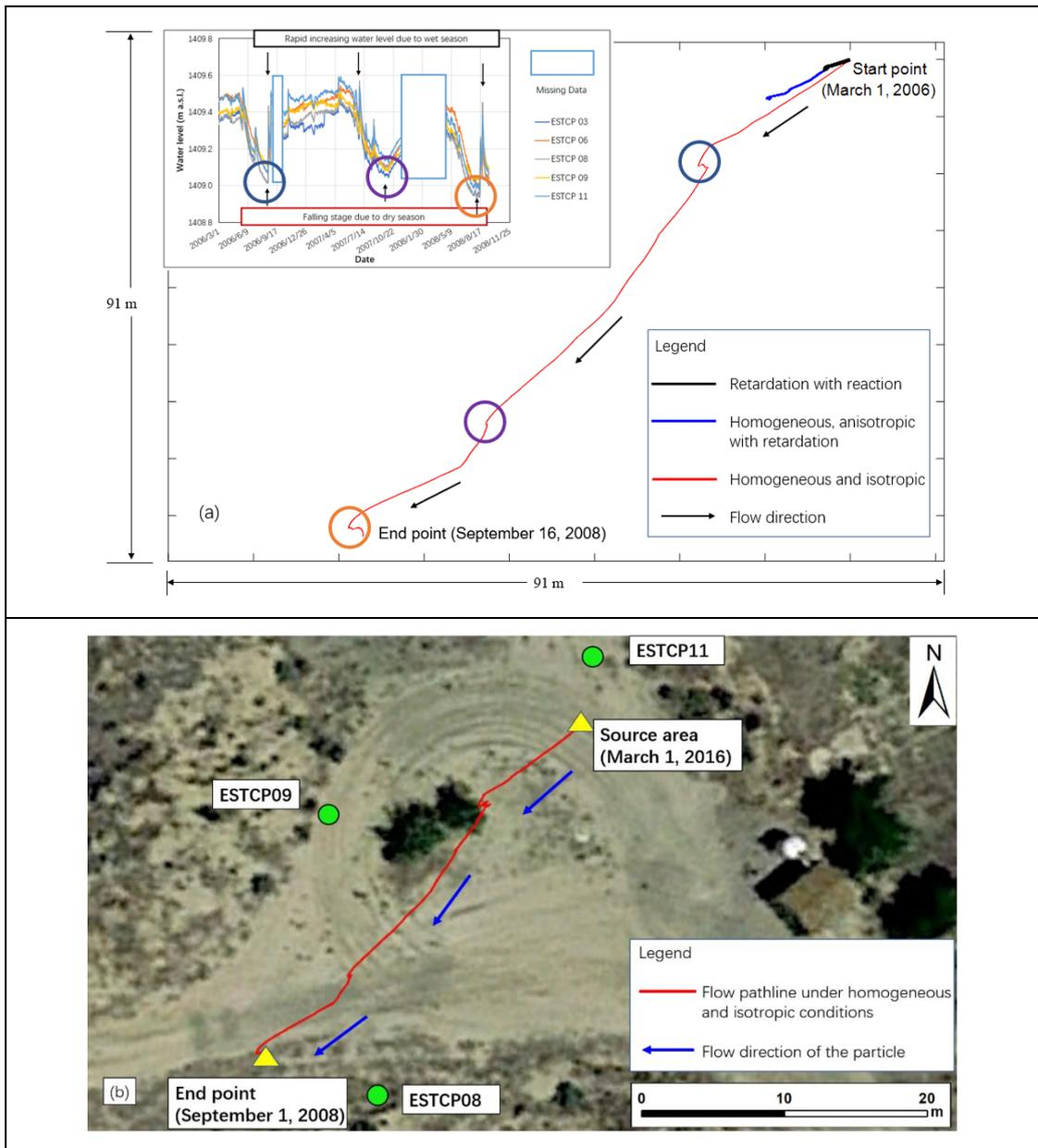
**Figure 6.** (a) Flow pathline of particle tracked under in different geologic conditions at Pueblo chemical depot in Pueblo, CO (circles with specific color correspond to flow direction reversals). (b) Flow pathline of particle tracked under homogeneous and isotropic conditions by assuming a source area at the study site.
