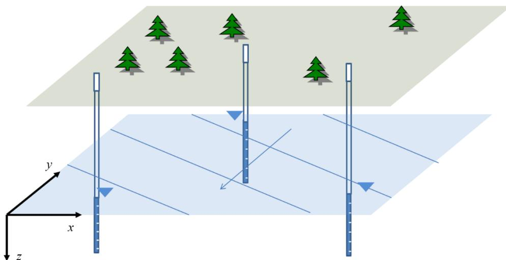
Figure 4. Three wells used to resolve the plane of the groundwater surface below an area of interest.
