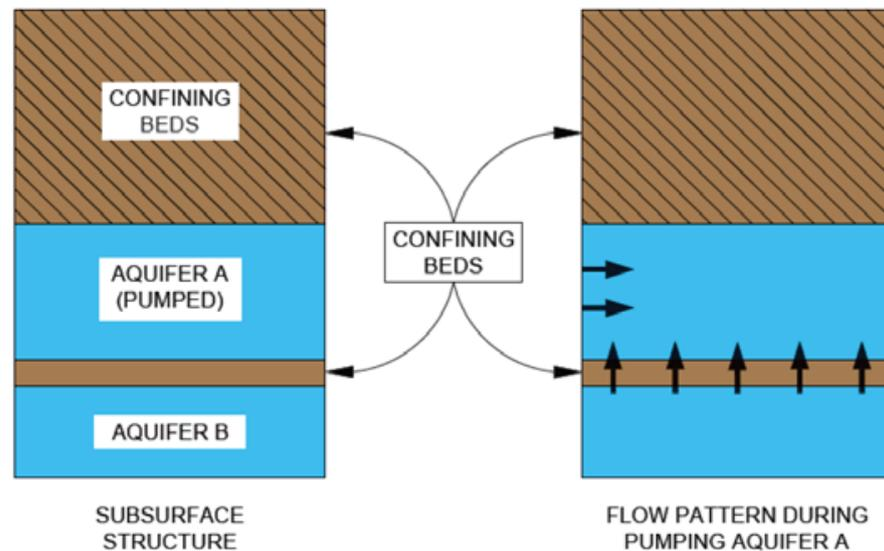
**Figure 1.** General conceptual model applied to wellfields being used to provide feedwater to BWRO plants in southern Florida (from Drendel et al. [20]).
