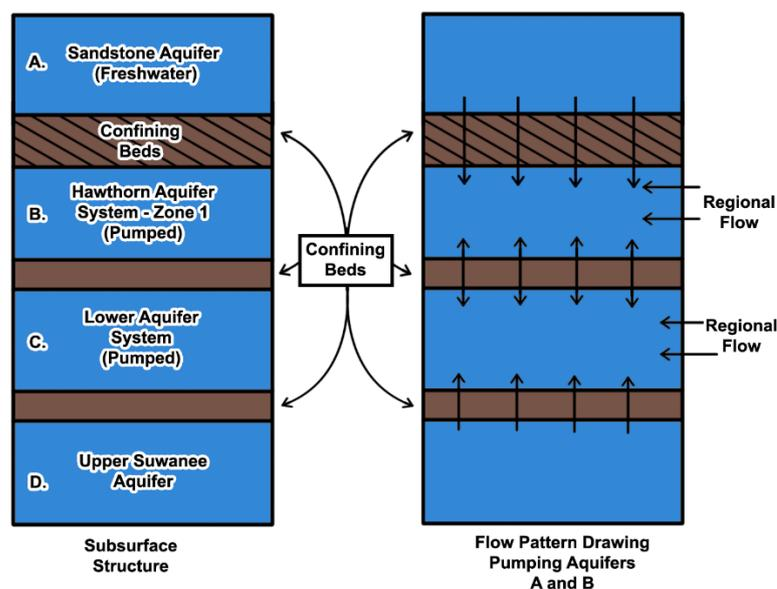
Figure 10. Conceptual model for the South Collier BWRO Plant Wellfield.
