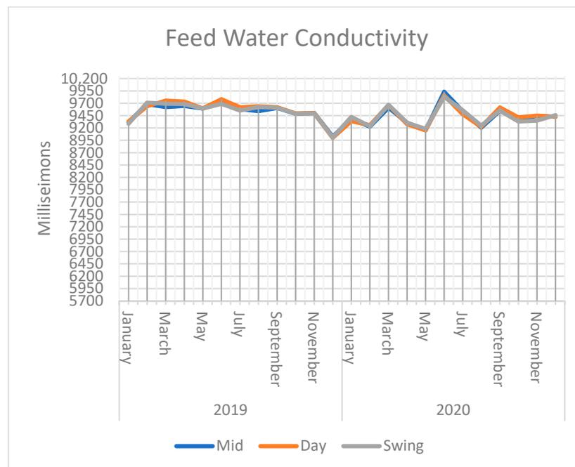
**Figure 11.** Conductivity of the feed water for 2019 and 2020. The mean is near 9400 milliseimens, which is an estimated TDS of 4700 mg/L or a dissolved chloride value of about 2585 mg/L.
