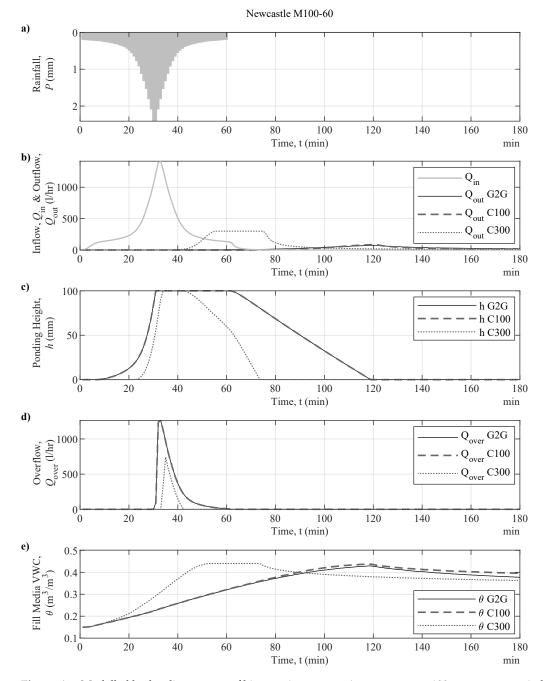
**Figure A2.** Modelled hydraulic response of bioretention systems in response to a 100-year return period 60-min duration storm event for Newcastle, UK. (a) Rainfall depth; (b) system inflow and outflow; (c) ponding height; (d) overflow; and (e) volumetric water content (VWC) of the fill media.
