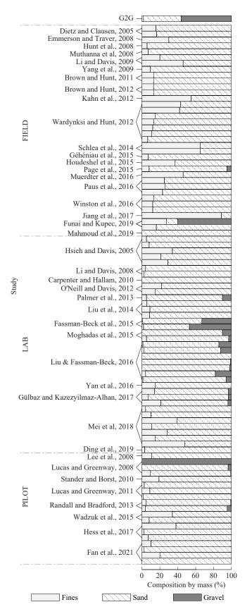
**Figure 5.** Comparison of G2G and literature examples of fill media composition by particle size class. Fines (<0.063 mm), sand (0.063–2.0 mm) and gravel (>2.0 mm).
