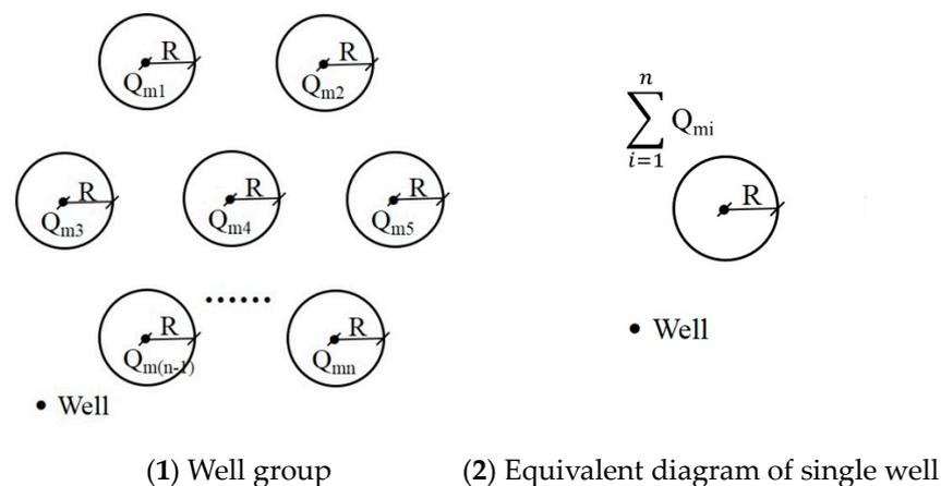
**Figure 4.** Influence radius in well group pumping and single well pumping in influence radius theory.  $R$  is the influence radius, [L];  $Q_{mi}$  is the maximum water yield of pumping well  $i$ , [ $L^3T^{-1}$ ]; and  $n$  is the number of pumping wells.
