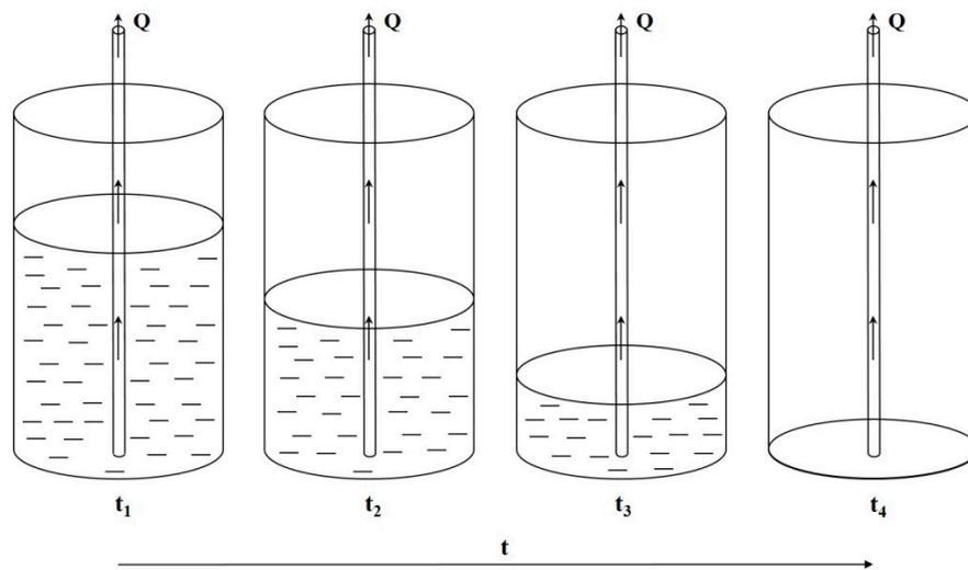
(1) Drawing water from cup (aquifer) without recharge (used as analogy for pumping in bounded aquifer).
