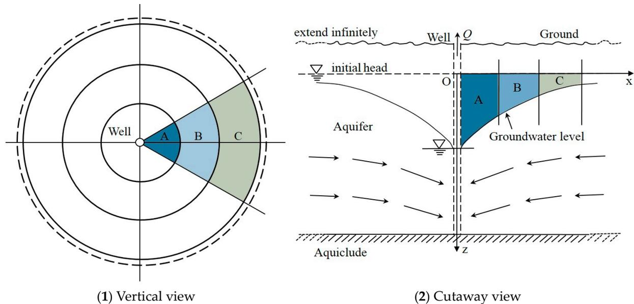
**Figure 6.** Formation of cone of depression of groundwater level during pumping.  $Q$  is the water yield of the pumping well,  $[L^3T^{-1}]$ .
