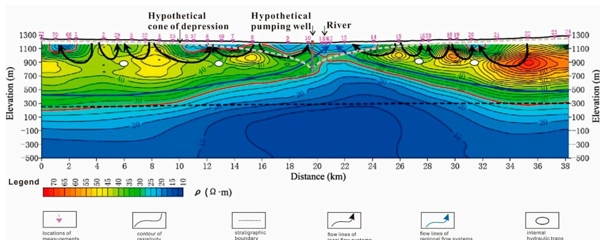
**Figure 5.** Schematic flow lines of a practical site according to the distribution of apparent resistivity, with a hypothetical pumping well added (modified from [27]).
