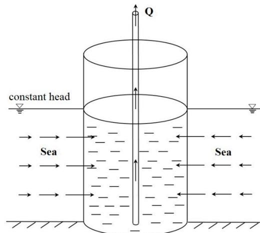
(2) Drawing water from cup (aquifer) with constant head on the side (used as analogy to Dupuit circular island model).
