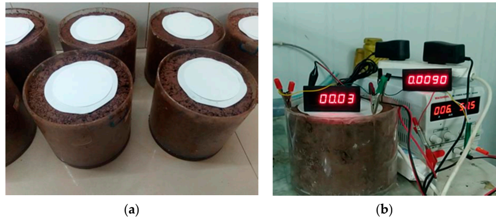
Figure 3. Sandstone specimen. (a) Substrate suction test; (b) electrical resistivity test.
