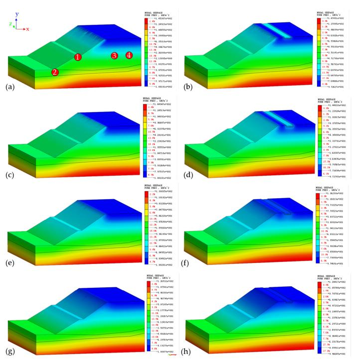
Figure 5 shows a cloud diagram of pore water pressure distribution of subgrade slope within 48 h after rainfall without and with bioretention facility.
