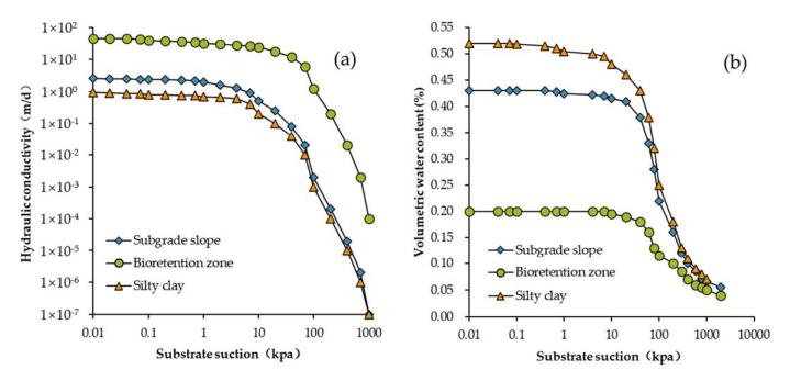
Figure 4. Hydraulic conductivity (a) and soil-water characteristic (b) curves of different materials.
