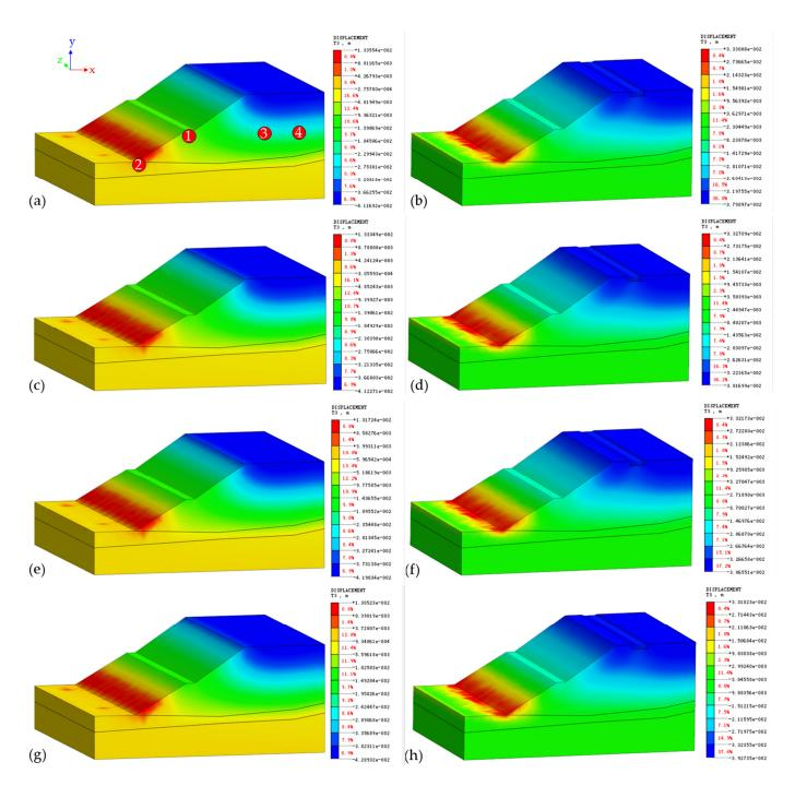
**Figure 10.** Comparison of vertical displacement distribution in subgrade slopes without or with biological retention facilities within 48 h after rainfall: (**a**,**b**) 6 h; (**c**,**d**) 12 h; (**e**,**f**) 24 h; (**g**,**h**) 48 h.
