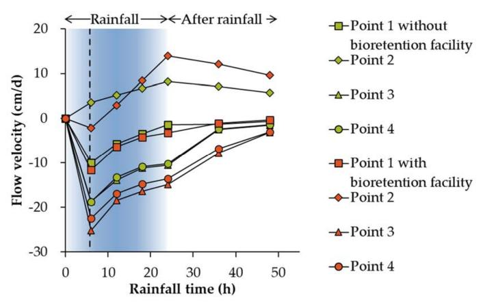
Figure 8. Flow velocity curves of different control points.
