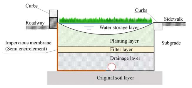
Figure 1. Cross-sectional view of road bioretention.
