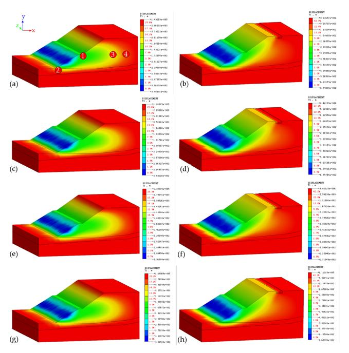
**Figure 9.** Comparison of horizontal displacement distribution in subgrade slopes without or with biological retention facilities within 48 h after rainfall: (**a**,**b**) 6 h; (**c**,**d**) 12 h; (**e**,**f**) 24 h; (**g**,**h**) 48 h.
