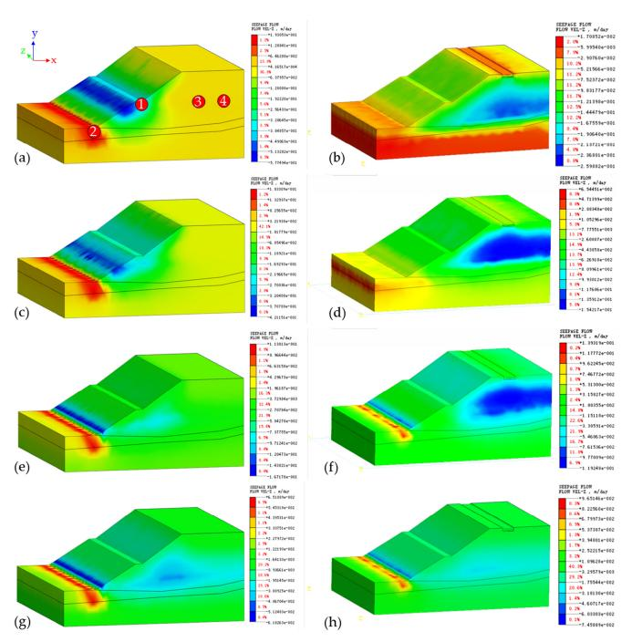
**Figure 7.** Comparison of water flow rate distribution in subgrade slopes without or with biological retention facilities within 48 h after rainfall: (**a**,**b**) 6 h; (**c**,**d**) 12 h; (**e**,**f**) 24 h; (**g**,**h**) 48 h.
