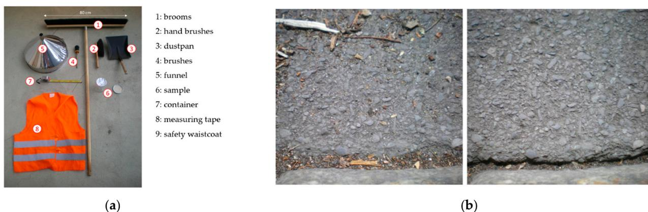
**Figure 2.** (a) RDS sample equipment (b) before/after close-up of a RDS sampling.
