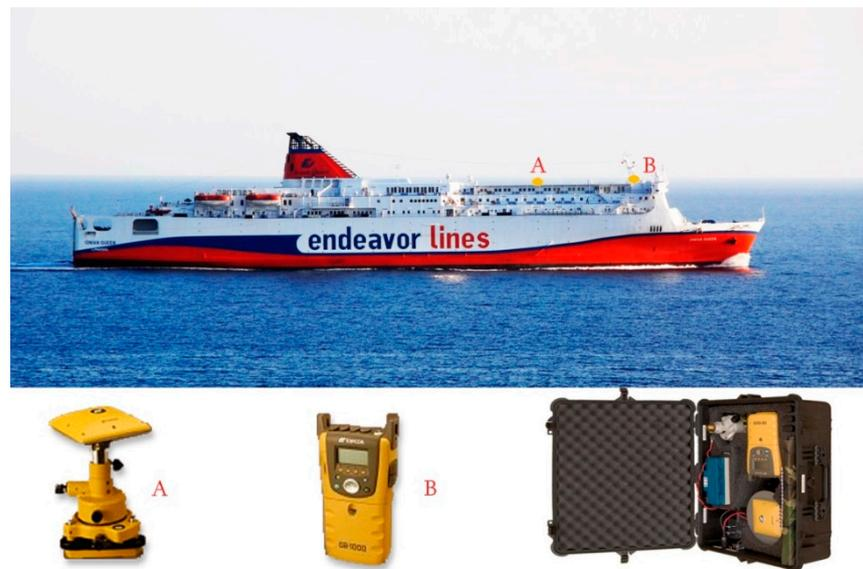
**Figure 2.** The “Ionian Queen” passenger ship used for the Ionian and Adriatic Sea measurements, and the basic Global Navigation Satellite System (GNSS) equipment. The antenna of the receiver was placed at point A with a tribrach in order to ensure leveling. The receiver was placed at point B in a special waterproof case for its protection.
