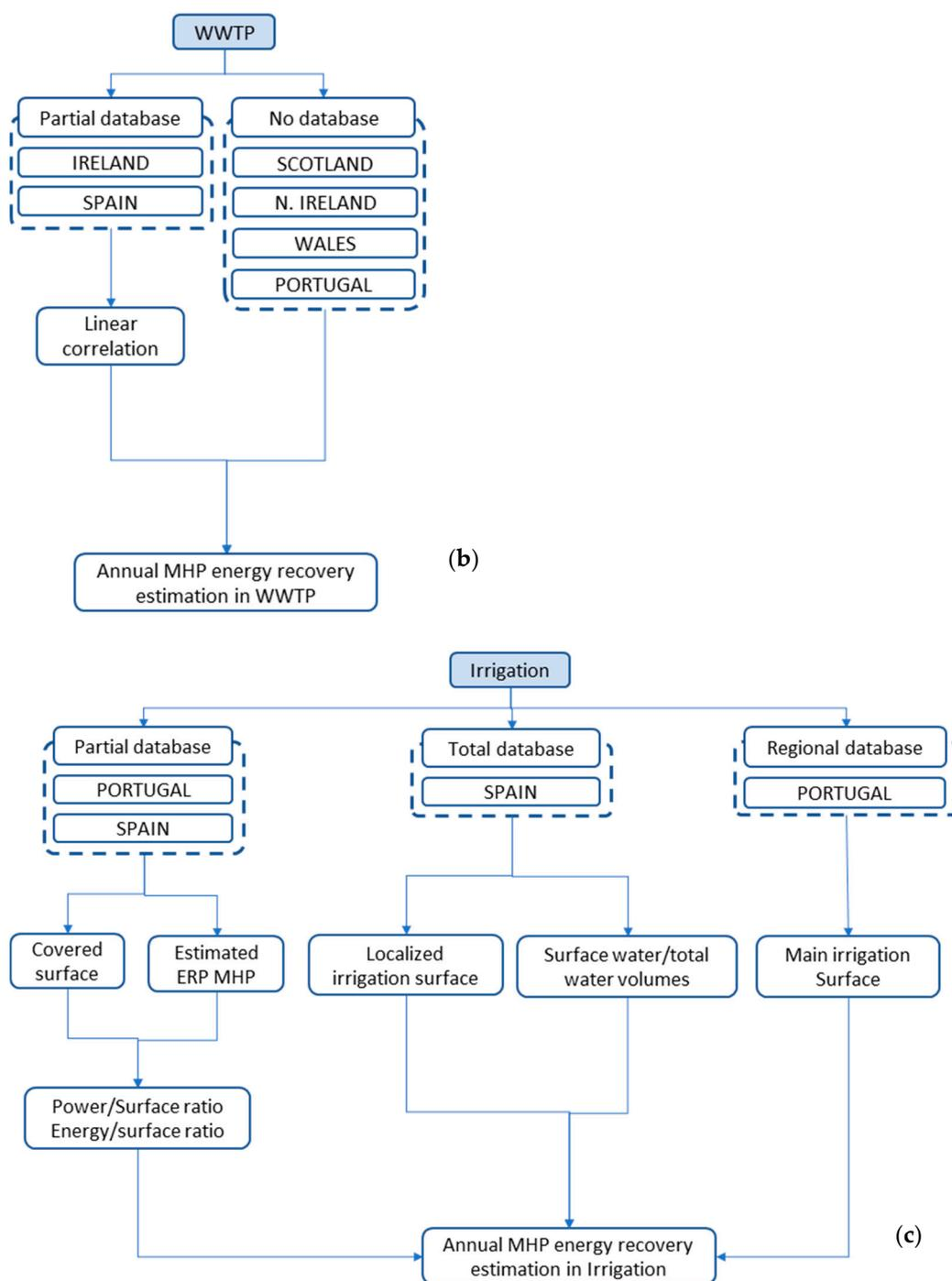
**Figure 2.** (a) Schematic representation of the methodology followed to estimate the MHP annual energy recovery potential (ERP) in the drinking water sector. (b) Schematic representation of the methodology followed to estimate the MHP annual energy recovery potential (ERP) in the wastewater sector. (c) Schematic representation of the methodology followed to estimate the MHP annual energy recovery potential (ERP) in the irrigation sector.
