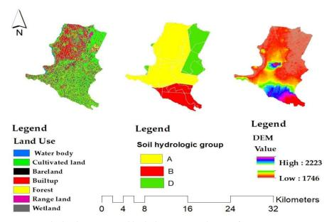
Figure 7. The land use map, soil hydrologic map and DEM of Hawassa City.
