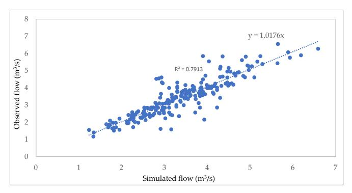
Figure 4. Best fit curve for flow calibration and validation.
