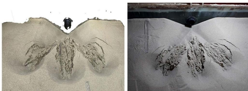
**Figure 3.** Three-dimensional dense point cloud in the software workspace (left) and real image of the sediment flushing cone (right).
