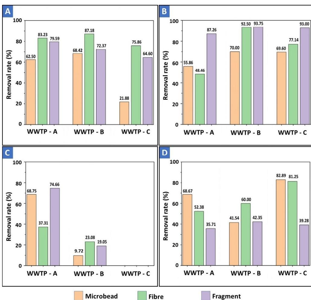
**Figure 5.** Removal efficiency of microplastic shapes at each treatment process. (A) Microplastic removal rate of screening and primary clarifier; (B) Microplastic removal rate of bioreactor and secondary clarifier; (C) Microplastic removal rate of coagulation; (D) Microplastic removal rate of disc-filter.
