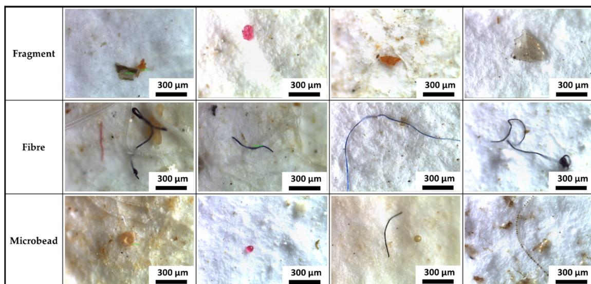
**Figure 3.** Result of microscope observation for microplastic particles.
