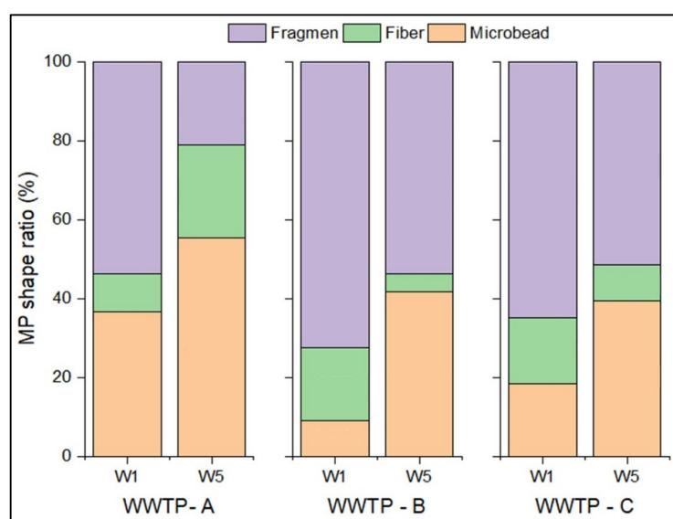
**Figure 4.** Comparison portion of microplastic shape between influent (W1) and effluent (W5).
