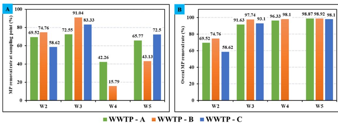
**Figure 2.** Removal of microplastic in different treatment processes. (A) Percentage of microplastics removed at sampling point; (B) Overall percentage of microplastic removal.
