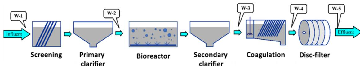
**Figure 1.** Sampling points and typical wastewater treatment process.
