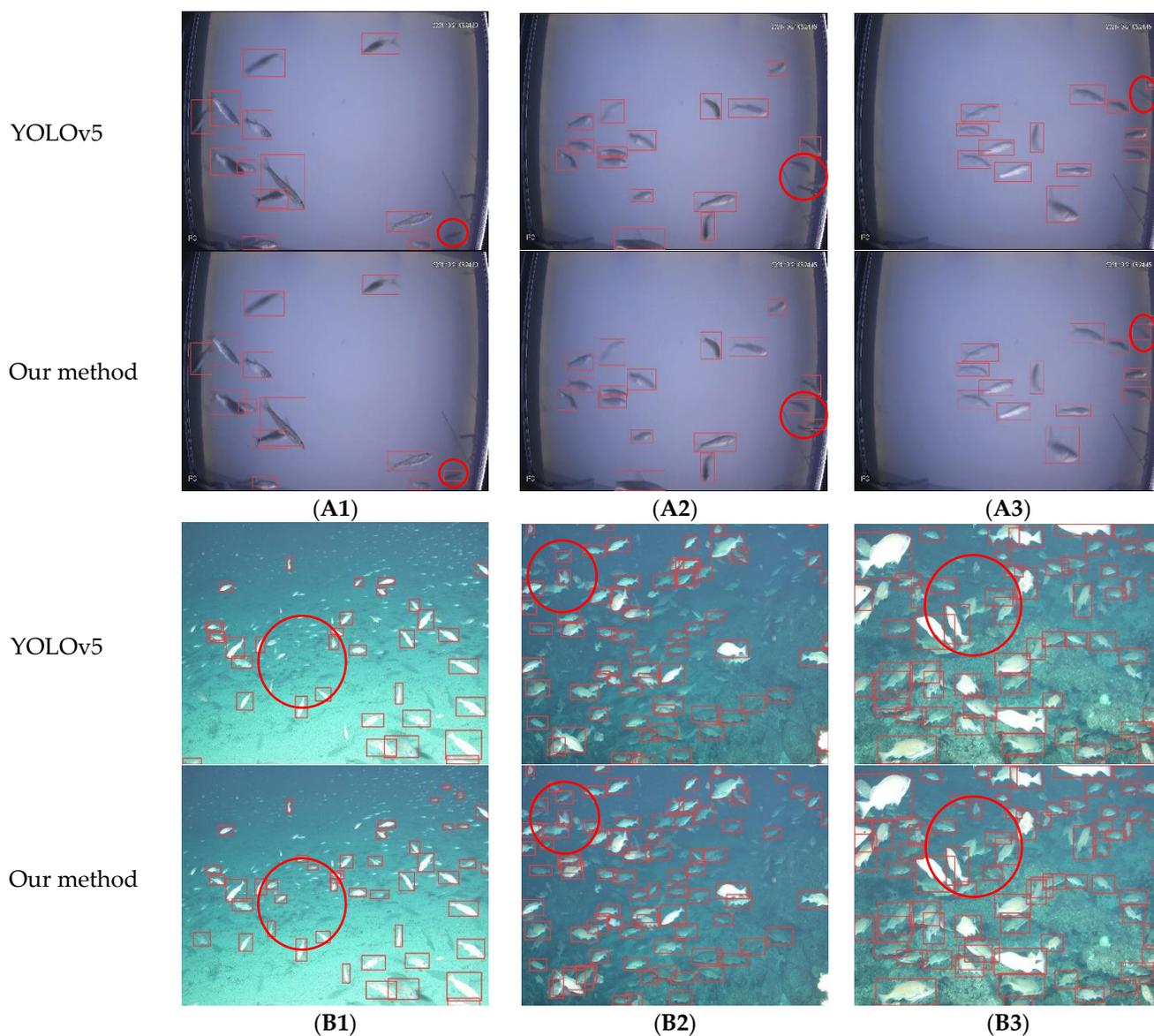
**Figure 4.** This is a figure showing the prediction results of the model: (A1) detection result of an occluded target in a power station image; (A2) detection result of a small target in a power station image; (A3) detection result of a fuzzy target in a power station image; (B1) small target fish image detection results; (B2) densely spaced fish and small target detection results; and (B3) fish and small target detection results under exposure.
