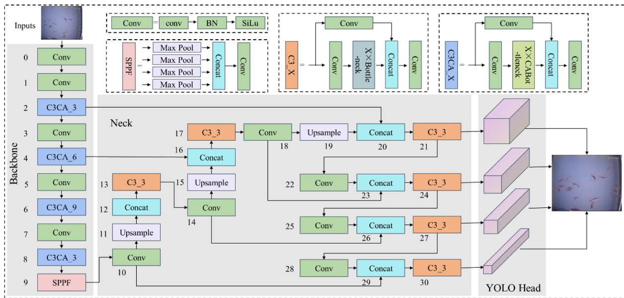
**Figure 1.** This is a figure that showing CME-YOLOv5 network structure. The numbers 1 to 30 in the figure represent the layers of the CME-YOLOV5 model.
