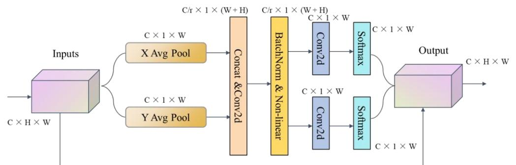
**Figure 2.** Schematic diagram of the CA mechanism module.
