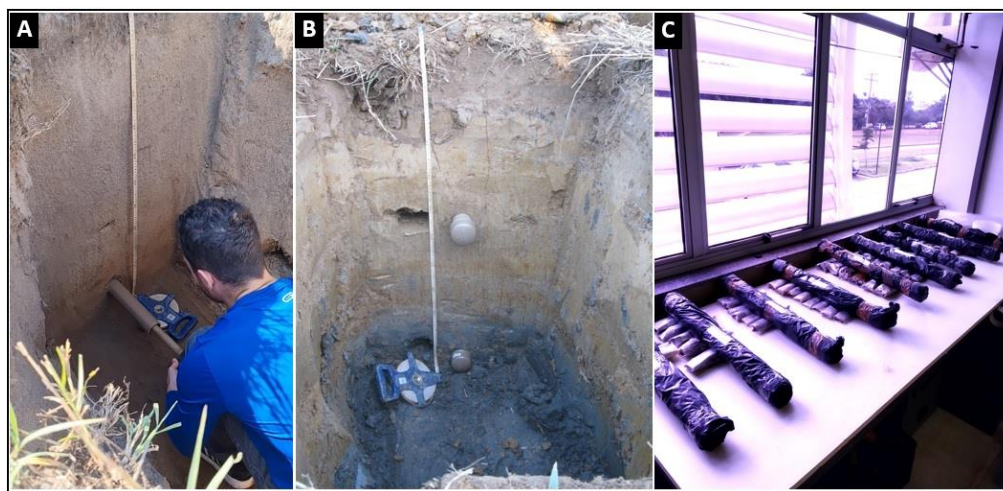
Figure 2. Example of sample collection procedure for OSL dating. (A) Horizontal introduction of the PVC pipe at a certain depth of interest after opening the trench; (B) Pipes inserted and capped, ready to be taken out of the trench; (C) Pipes sealed in the laboratory ready to be sent for dating by OSL. (Photo by: L. Lämmle, April/2021).
