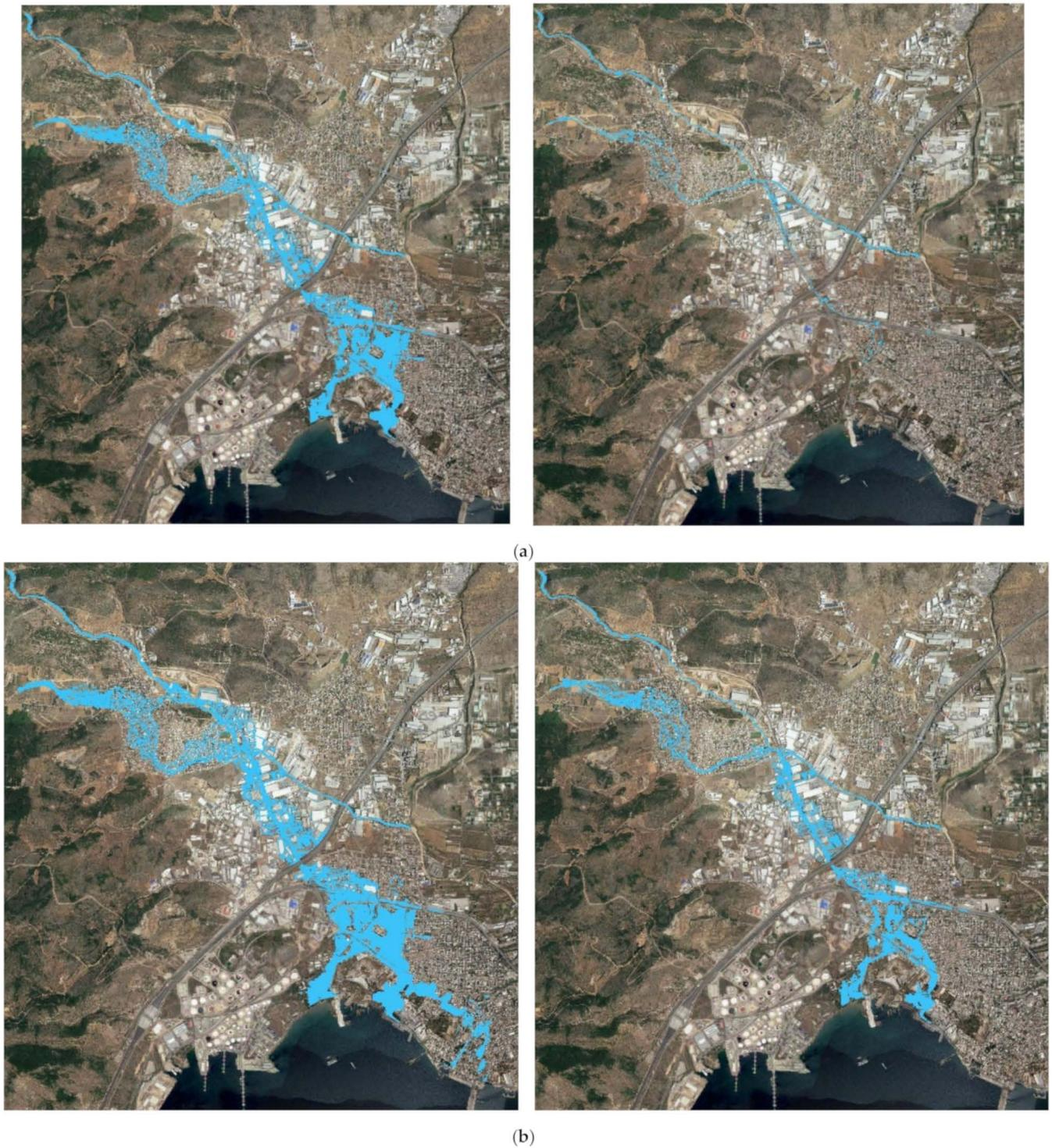
**Figure 4.** Inundation area for 4 indicative scenarios: (a) Scenarios S20-06 (left) and W20-06 (right) for  $T = 20$  y and  $t = 6$  h. (b) Scenarios S200-18 (left) and W200-18 (right) for  $T = 200$  y and  $t = 18$  h.
