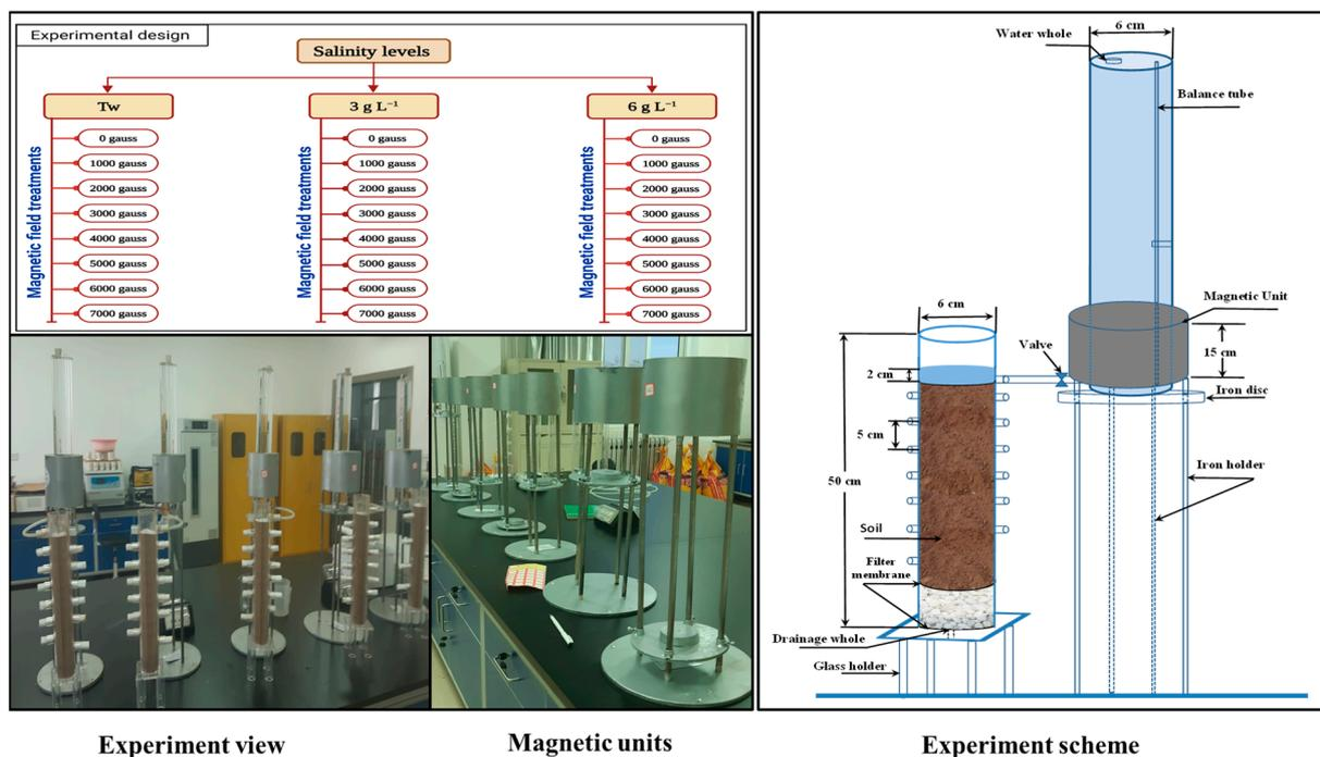
**Figure 1.** Experimental design, photos of the experiments, and a schematic representation of the experimental system.
