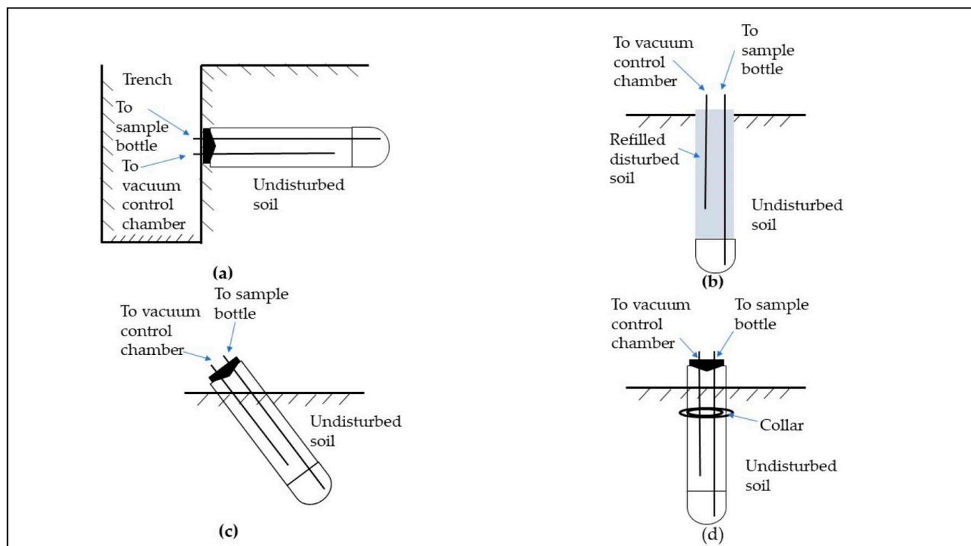
**Figure 2.** Different installation methods with tension lysimeters: (a) horizontal installation, (b) vertical without shaft, (c) vertical at 45°, and (d) vertical with the collar.
