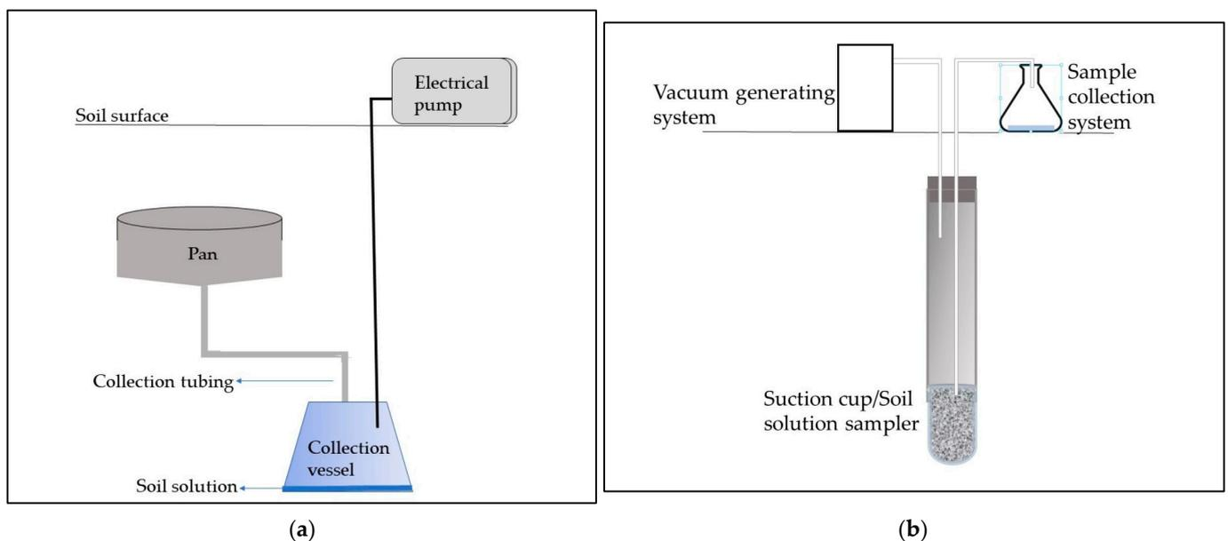
**Figure 1.** Schematic diagrams of zero-tension and tension lysimeters: (a) zero-tension lysimeter; (b) tension lysimeter.
