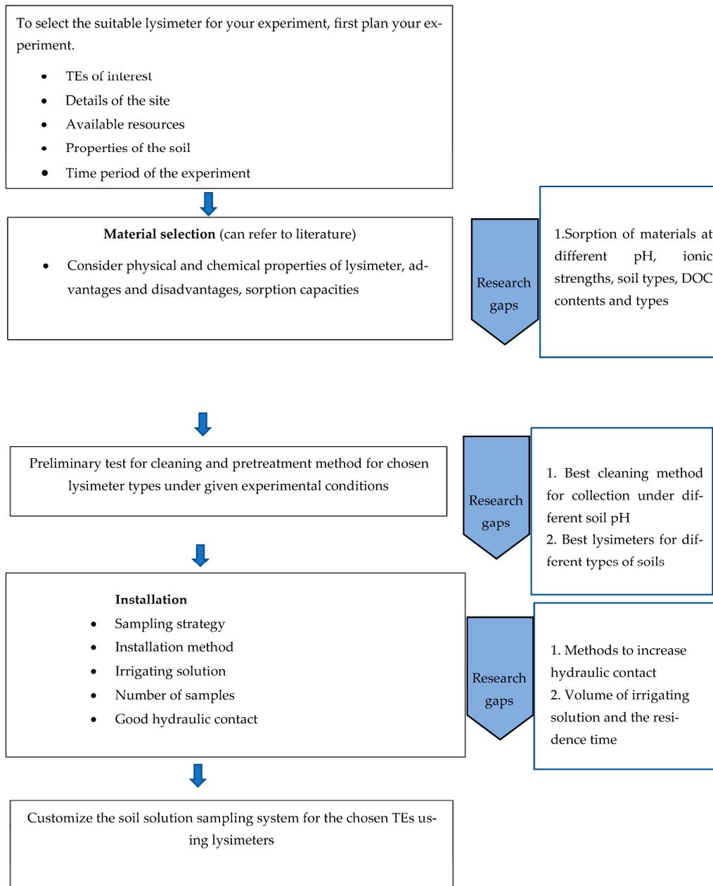
Figure 3. Flow chart to optimize lysimeter sampling system for specific experimental conditions.
