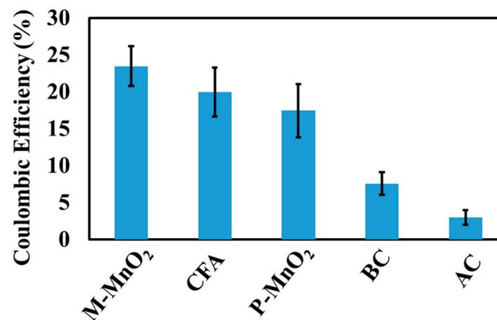
Figure 5. Average CE efficiency values with deviations of the five units with the different cathode assemblies (P-MnO<sub>2</sub>, M-MnO<sub>2</sub>, CFA, BC, AC) versus time.
