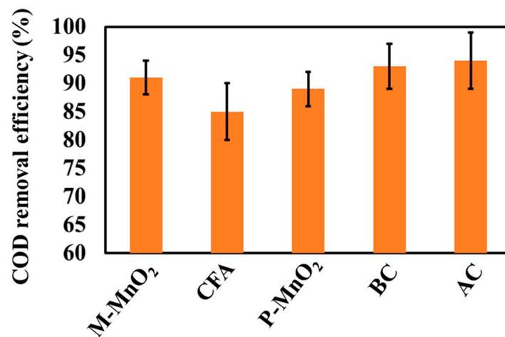
Figure 4. Average COD removal efficiency values with deviations of the five units with the different cathode assemblies (P-MnO<sub>2</sub>, M-MnO<sub>2</sub>, CFA, BC, AC) versus time.
