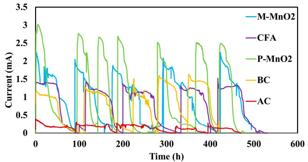
Figure 3. Current output during consecutive batch experiments of the five units with the different cathode assemblies (P-MnO<sub>2</sub>, M-MnO<sub>2</sub>, CFA, BC, AC) versus time.
