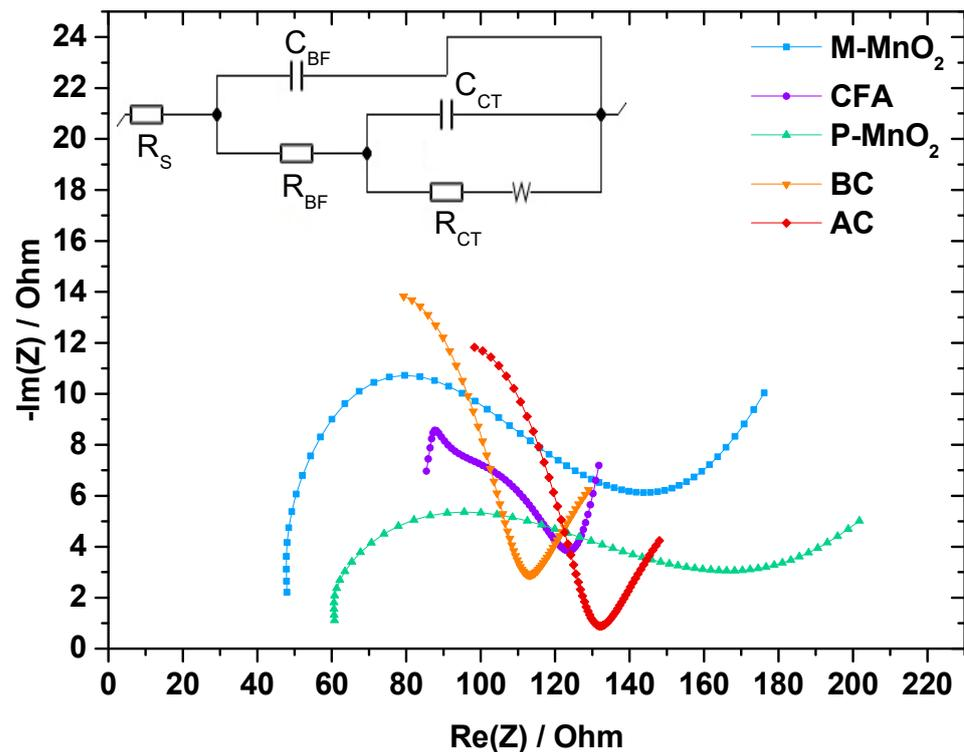
Figure 7. Nyquist (Bode-Bode) plots from EIS measurements.
