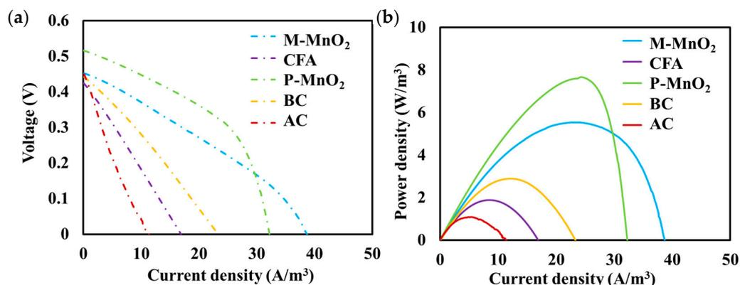
**Figure 6.** MFC voltage  $U_{\text{cell}}$  (a) and power density (b) versus current density for the different cathode strategies (P-MnO<sub>2</sub>, M-MnO<sub>2</sub>, CFA, BC, AC).
