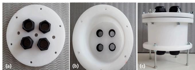
**Figure 1.** Photos of (a) the top lid, (b) the internal view and (c) the MFC units.
