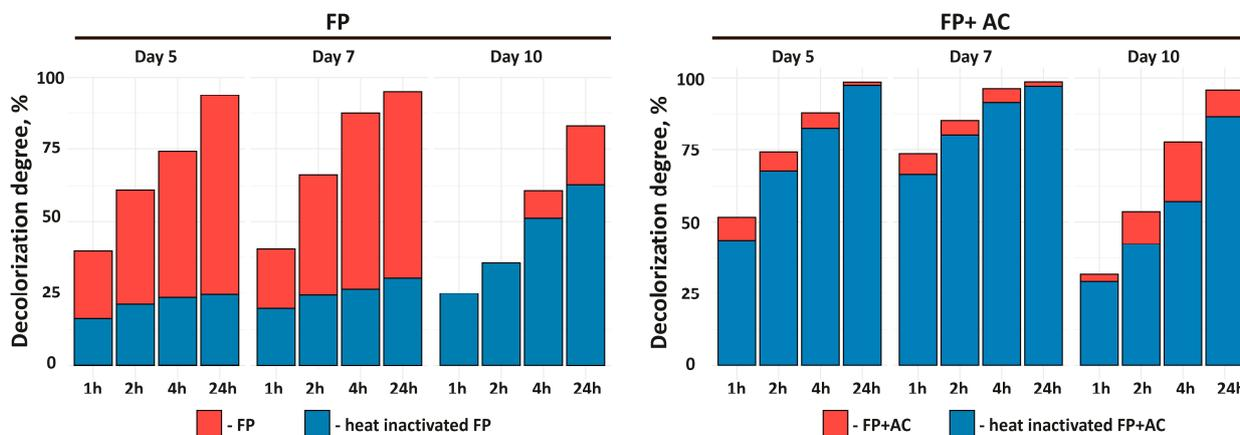
**Figure 3.** The decolorization of RBBR (with a starting concentration of 50 μM) by fungal pellets (FP) and fungal pellets supplemented with activated carbon (FP+AC) that were collected on the 5th, 7th, and 10th day of *T. hirsuta* cultivation.
