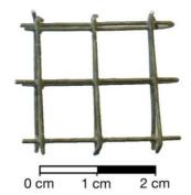
Figure 1. Galvanised wire cage used in modifications to the Alka-Seltzer test.
