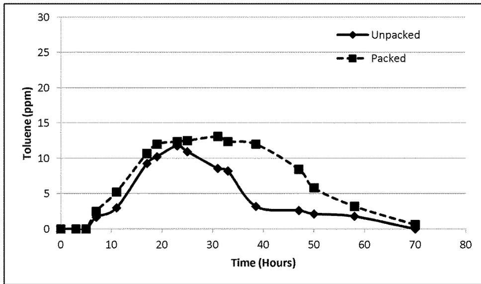
**Figure 4.** Toluene degradation results for packed system.
