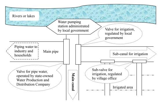
Figure 2. Surface water distributions between irrigation water and pipe water.
