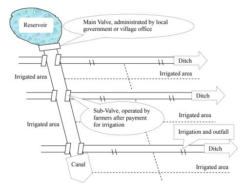
Figure 3. Reservoir irrigation systems at village level.
