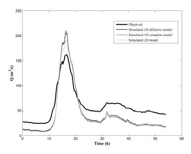
**Figure 8.** Comparison between observed and computed discharge hydrographs at Europa Bridge site for the 1D models and the 2D model ('soft' data).
