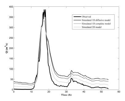
**Figure 9.** Comparison between observed and computed discharge hydrographs at Castiglione Scalo site for the 1D models and the 2D model ('soft' data).
