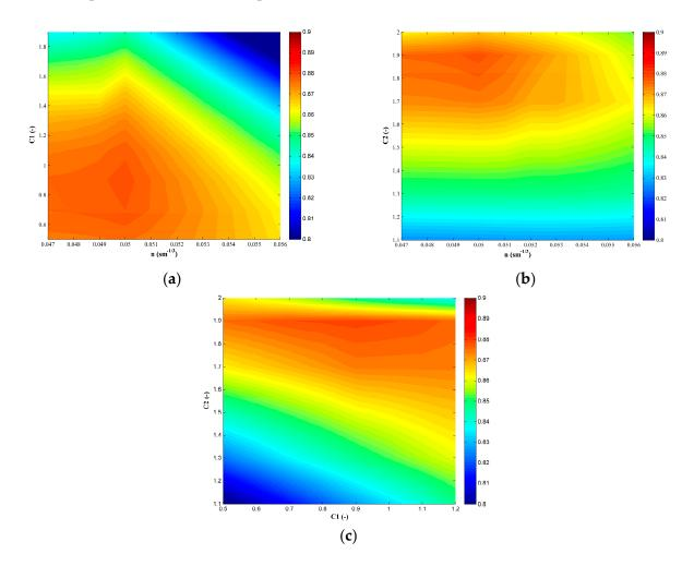
**Figure 6.** Castiglione Scalo section, 1D diffusive model: Nash Sutcliffe, NSh, versus: (a)  $C_1$  and n parameters for fixed optimum  $C_2$  parameter; (b)  $C_2$  and n parameters for fixed optimum  $C_1$  parameter; (c)  $C_1$  and  $C_2$  parameters for fixed optimum n parameter.
