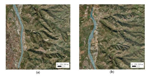
**Figure 7.** Inundated area computed by the 2D model (**a**) at Europa bridge site and (**b**) at Castiglione Cosentino site.
