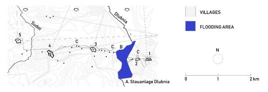
**Figure 6.** Reconstruction of the Dłubnia inundation area for the state from 1915. The watercourse was blocked by an improvised blockade under a bridge clearance. The water flowing downstream (due south) spilled successively into the river valley. Markings: A. location of the levee, B. inundation area, C. wire obstacle strip; 1. Fort Dłubnia, 2. Earthwork 1/Dłubnia, 3. Fort Mistrzejowice, 4. Fort Batowice, and 5. Fort Sudół. The expected avenues of attack are marked with arrows.
