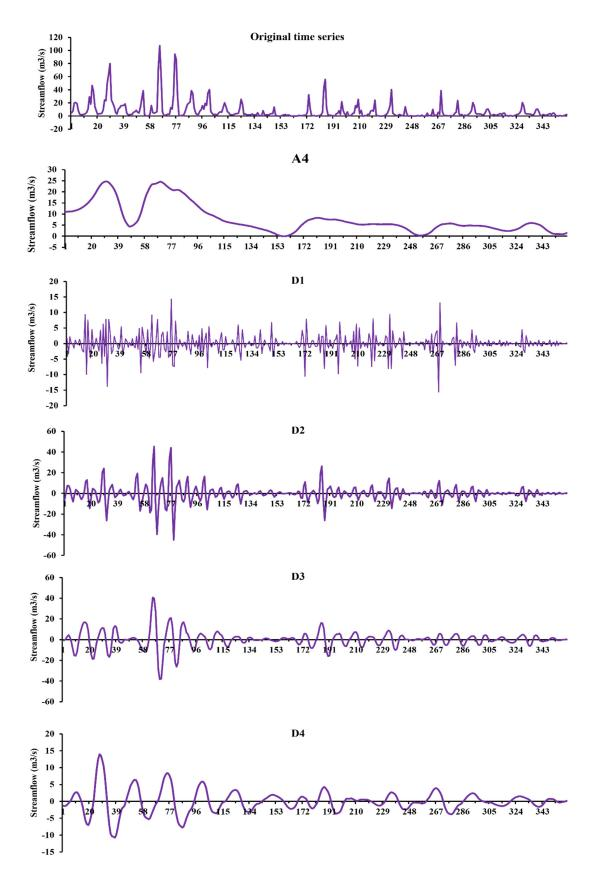
**Figure 3.** The approximation (A4) and detail (D1–D4) components of the monthly streamflow time series in the Akhola station.
