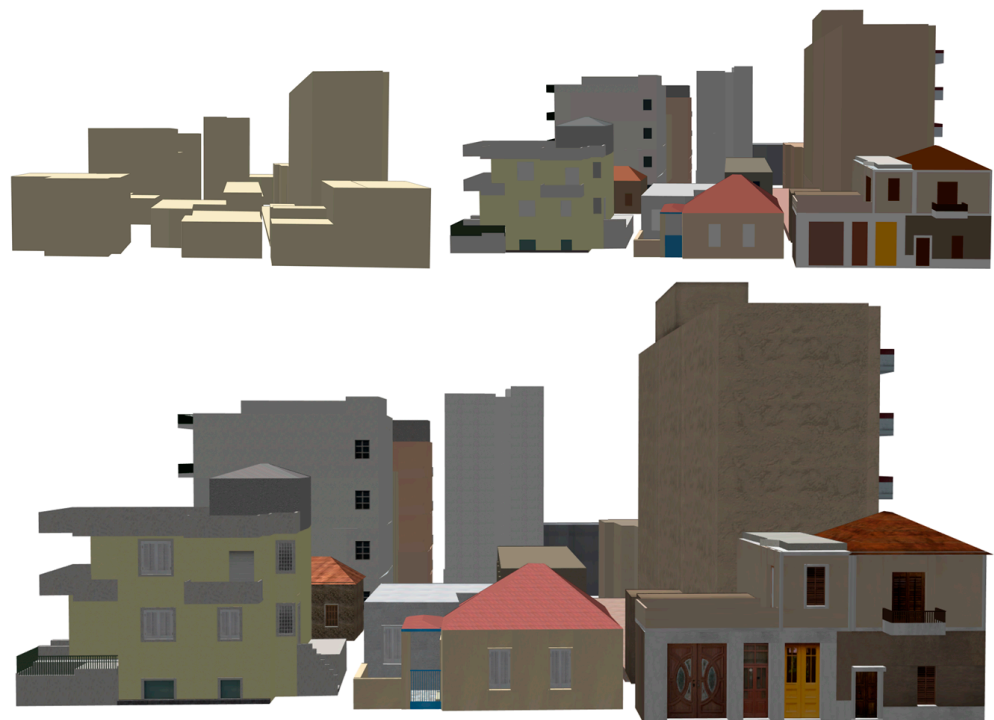
Figure 3. 3D views of the building models at LoD1 (top-left), LoD2 (top-right) and LoD3 (bottom).
