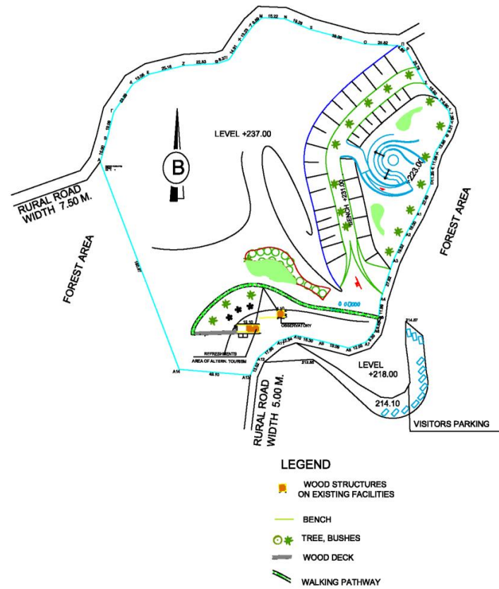
Figure 12. Restoration proposals for the quarry in Mikro Derio according to the alternative scenario A4, scale 1:2000.
