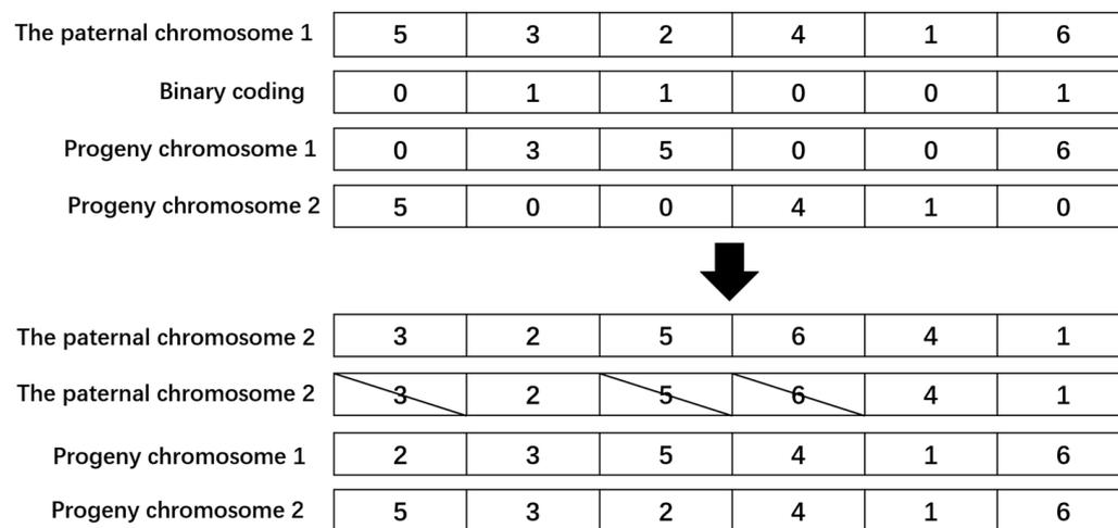
Figure 7. The uniform sort crossover operator of the stacking site.
