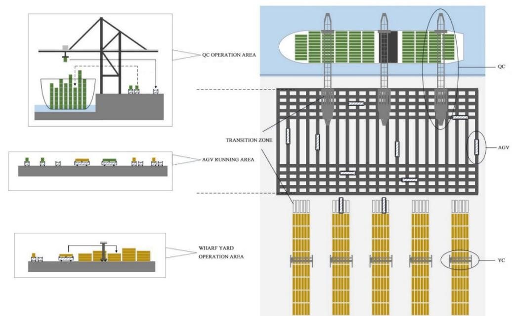
**Figure 1.** Automatic container terminal layout.
