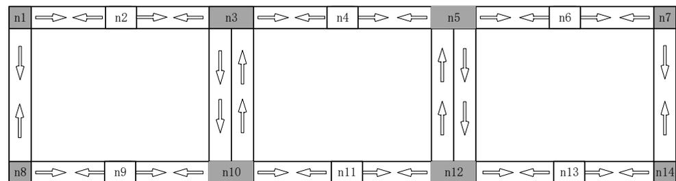
Figure 2. AGVs running path.
