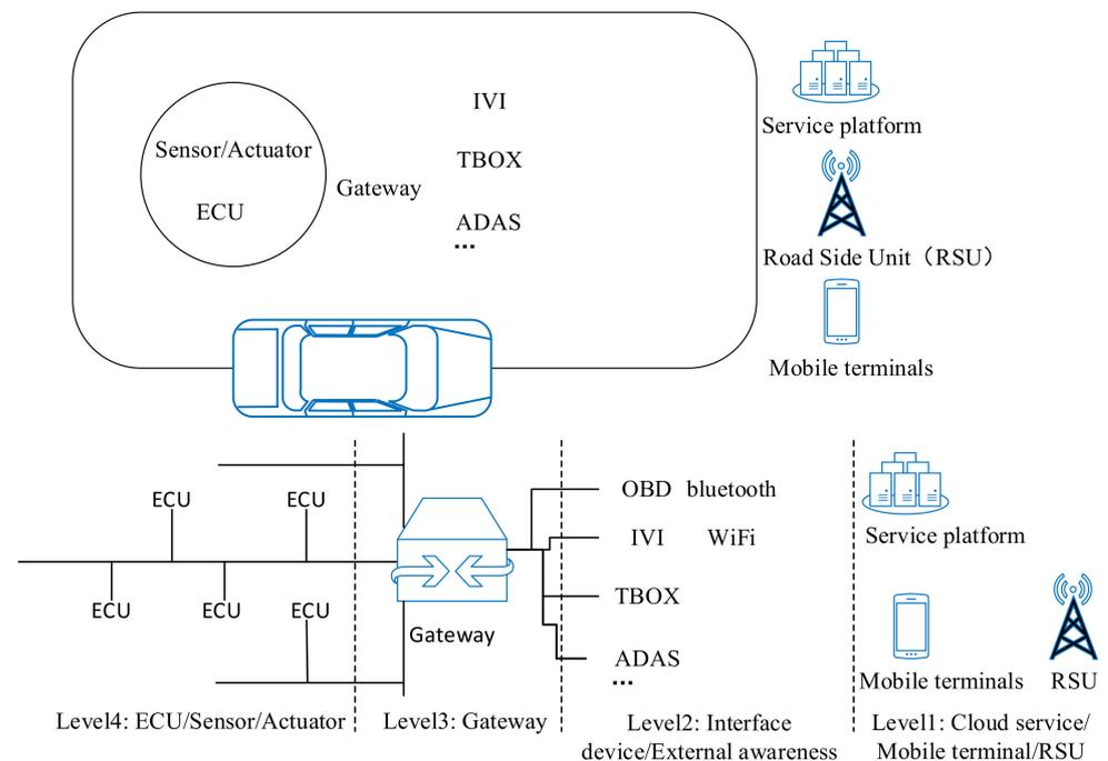
**Figure 1.** In-vehicle network security architecture.
