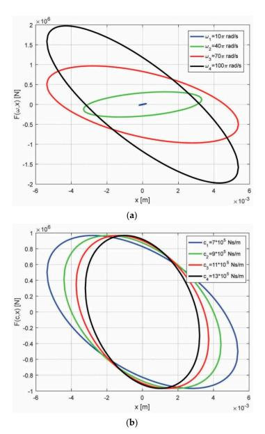
**Figure 7.** (a) Hysteresis loops F-x for  $F_0 = m_0 \text{r} \omega^2$ —discrete variation of  $\omega$  ( $m_0 r = 5$  kgm, m = 10,000 kg). (b) Hysteresis loops F-x for  $F_0 = m_0 \text{r} \omega^2$ —discrete variation of c ( $m_0 r = 5$  kgm, m = 10,000 kg).
