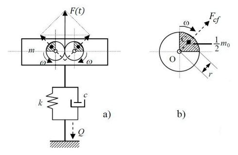
**Figure 1.** Scheme of the linear dynamic system (MCK) excited with force  $F(t) = m_0 r \omega^2 sin(\omega t)$ , where  $F_0 = F_0(\omega) = m_0 r \omega^2$  (a) Voigt–Kelvin model dynamic system; (b) eccentric body of the dynamic imbalance with mass  $\frac{1}{2}m_0$  and eccentricity r, in relation to the axis of rotation, with normal passing through O.
