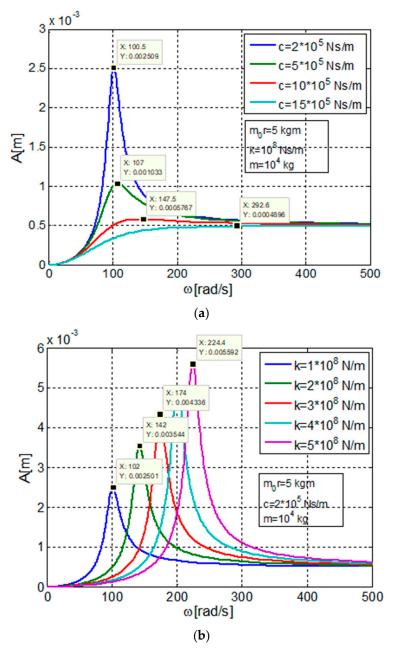
**Figure 2.** (a) The amplitude of steady-state vibration in dynamic regime—variation of amplitude function of  $\omega$  and c; (b) The amplitude of steady-state vibration in dynamic regime—variation of amplitude function of  $\omega$  and k.
