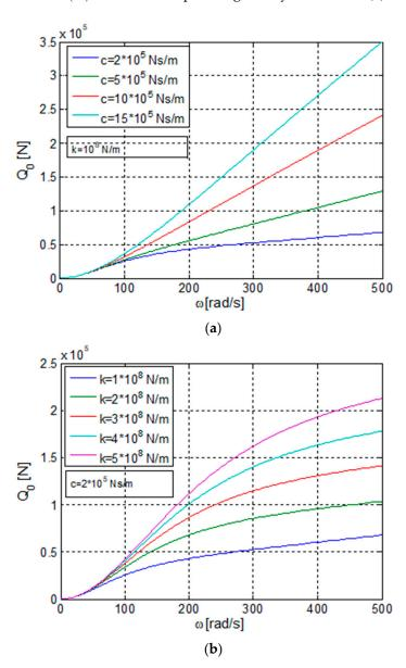
**Figure 3.** The amplitude of the transmitted force (maximum transmitted force). (a) The amplitude of the transmitted force  $Q_0$  function of  $\omega$  and c; (b) The amplitude of the transmitted force  $Q_0$  function of  $\omega$  and k.
