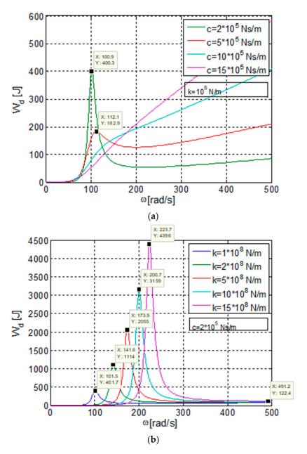
**Figure 6.** (a) Dissipated energy function of  $\omega$  and c (at constant stiffness k); (b) dissipated energy function of  $\omega$  and k (at constant damping c).
