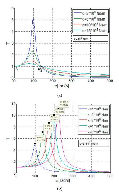
**Figure 5.** Transmissibility T = |T| (a) variation of T function of  $\omega$  and c; (b) variation of T function of  $\omega$  and k.
