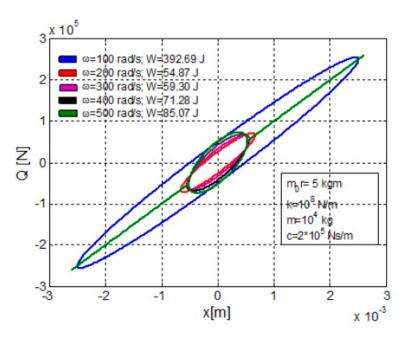
**Figure 4.** Hysteresis loops Q-x for the discrete variation of  $\omega$ .
