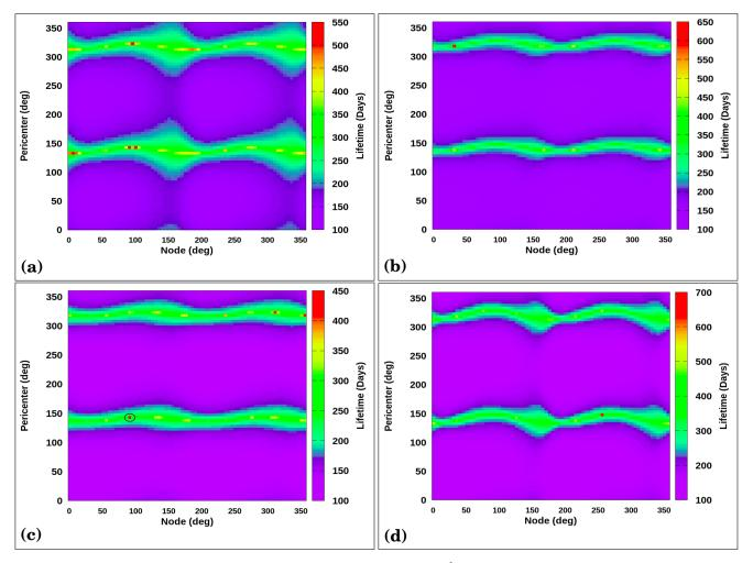
**Figure 7.** Diagram of  $\omega \times \Omega$  for  $e = 10^{-2}$  considering the effects of third-body and  $J_2$  and  $C_{22}$  of Titania: (a) a = 1000 km,  $I = 70^{\circ}$ ; (b) a = 1000 km,  $I = 80^{\circ}$ ; (c)  $I = 80^{\circ}$ , a = 1162 km; (d)  $I = 80^{\circ}$ , a = 914 km;  $\omega = 0-360^{\circ}$ ,  $\Omega = 0-360^{\circ}$ .
