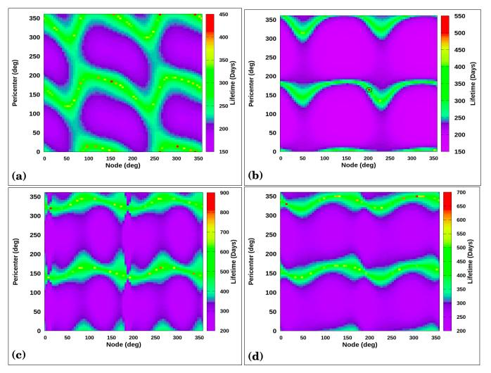
**Figure 5.** Diagram of  $\omega \times \Omega$  for  $e = 10^{-3}$  considering the effects of third-body and  $J_2$  and  $C_{22}$  of Titania: (a) a = 1265 km,  $I = 70^{\circ}$ ; (b) a = 1265 km,  $I = 80^{\circ}$ ; (c)  $I = 80^{\circ}$ , a = 834 km; (d)  $I = 80^{\circ}$ , a = 1000 km;  $\Omega = 0^{\circ} - 360^{\circ}$ ,  $\omega = 0^{\circ} - 360^{\circ}$
