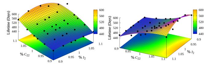
interaction term between  $J_2$  and  $C_{22}$ , the function provides a good approximation of the lifetime as a function of the percentage values of Titania's gravitational coefficients.
