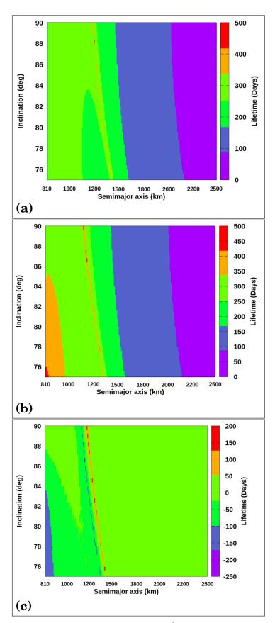
**Figure 2.** Diagram of *a* versus *I* for  $e = 10^{-3}$ : (a) considering only the effects from Uranus; (b) including the third-body and the effects of  $J_2$  and  $C_{22}$  of Titania; (c) lifetime differences (third body  $-J_2$  and  $C_{22}$  of Titania). Initial values are a = 810-1200 km,  $I = 75-90^\circ$ ,  $\omega = 0^\circ$ , and  $\Omega = 0^\circ$ .
