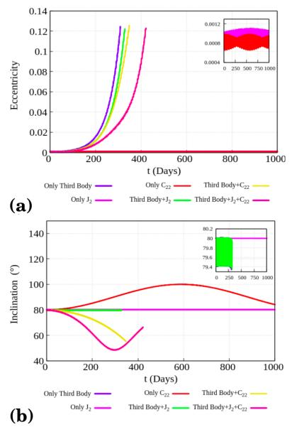
**Figure 9.** Diagram of  $e \times t$  and  $I \times t$  showing different perturbative effects: considering only the perturbations by Uranus, only  $J_2$  from Titania, only  $C_{22}$  from Titania, Uranus  $+J_2$  from Titania, Uranus  $+C_{22}$  from Titania, and Uranus  $+J_2 + C_{22}$  from Titania. Initial values are  $a_i = 900$  km,  $e_i = 10^{-3}$ ,  $I_i = 80^\circ$ ,  $\omega_i = \Omega_i = 0^\circ$ .
