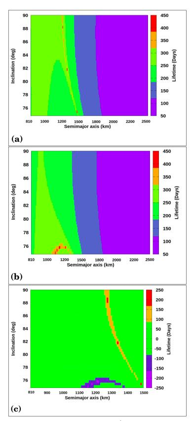
**Figure 8.** Diagram of *a* versus *I* for  $e = 10^{-2}$ : (a) considering only the effects from Uranus; (b) including third-body and effects from  $J_2$  and,  $C_{22}$  of Titania; (c) lifetime differences (third body  $-J_2$  and  $C_{22}$  of Titania). Initial values ares a = 810-1500 km,  $I = 75-90^\circ$ ,  $\omega = 145^\circ$ , and  $\Omega = 95^\circ$ .
