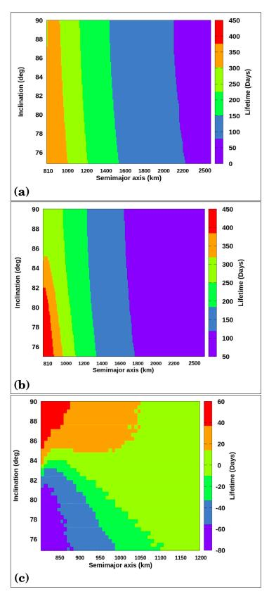
**Figure 1.** Diagram of *a* versus *I* for e = 0: (a) considering only the effects from Uranus; (b) including the third-body and the effects of  $J_2$  and  $C_{22}$  of Titania; (c) lifetime differences (third body  $-J_2$  and  $C_{22}$  of Titania). Initial values are a = 810-1200 km,  $I = 7-90^{\circ}$ ,  $\omega = 0^{\circ}$ , and  $\Omega = 0^{\circ}$ .
