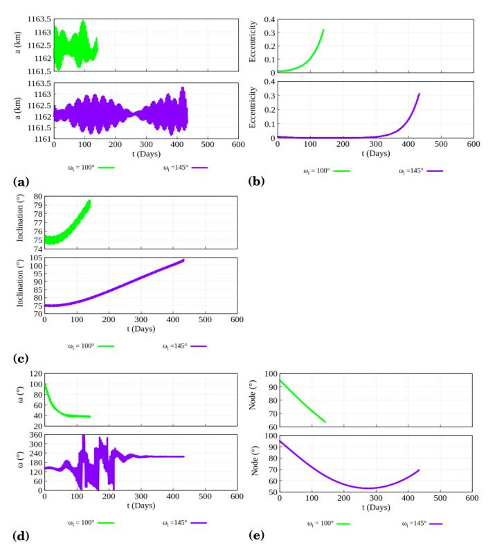
**Figure 11.** Temporal evolution of the orbital elements considering  $\omega = 100^{\circ}$  and  $\omega = 145^{\circ}$ : (a)  $a \times t$ , (b)  $e \times t$ , (c)  $I \times t$ , (d)  $\omega \times t$ , and (e)  $\Omega \times t$ . Initial conditions are  $a_i = 1162$  km,  $e_i = 10^{-2}$ ,  $I_i = 75^{\circ}$ ,  $\Omega_i = 95^{\circ}$ . In these figures the effects considered are the perturbation by Uranus,  $+J_2$  and  $C_{22}$  of Titania.
