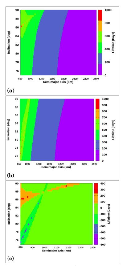
**Figure 6.** Diagram of *a* versus *I* for  $e = 10^{-3}$ : (a) considering only the effects from Uranus; (b) including the third-body and the effects of  $J_2$  and  $C_{22}$  of Titania; (c) lifetime differences (third body  $-J_2$  and  $C_{22}$  of Titania). Initial values are a = 810-1400 km,  $I = 75-90^{\circ}$ ,  $\omega = 165^{\circ}$ , and  $\Omega = 205^{\circ}$ .
