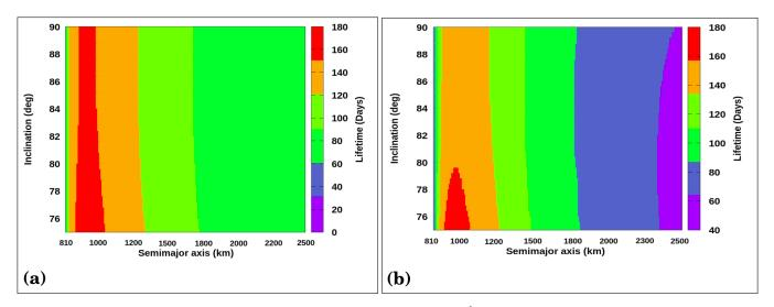
**Figure 3.** Diagram of *a* versus *I* for  $e = 10^{-2}$ : (a) considering only the effects from Uranus; (b) including the third-body and the effects of  $J_2$  and  $C_{22}$  of Titania. Initial values are a = 810-2500 km,  $I = 75-90^{\circ}$ ,  $\omega = 0^{\circ}$ , and  $\Omega = 0^{\circ}$ .
