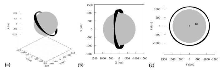
**Figure 12.** Trajectory numerically simulated for 991 days, considering the complete system, the gravitational effects of the third body (Uranus), and Titania's gravitational coefficients ( $J_2$  and  $C_{22}$ ). (a) Projection of the orbit in three dimensions (xyz). (b) Projection of the orbit in the plane (xy). (c) Projection of the orbit in the plane (yz). The initial conditions are: a = 898 km,  $e = 10^{-3}$ ,  $I = 81.4^{\circ}$ ,  $\omega = 140^{\circ}$ , and  $\Omega = 225^{\circ}$ .
