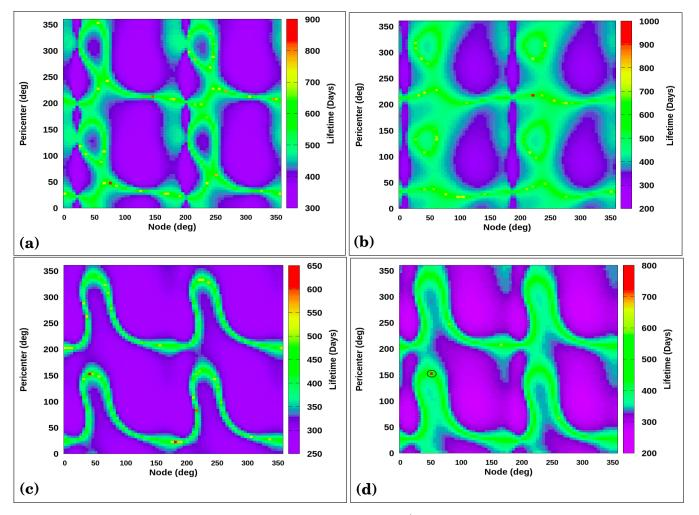
**Figure 4.** Diagram of  $\omega \times \Omega$  for  $e = 10^{-4}$  considering the effects of third-body and  $J_2$  and  $C_{22}$  of Titania: (a) a = 900 km,  $I = 70^{\circ}$ ; (b) a = 900 km,  $I = 80^{\circ}$ ; (c)  $I = 80^{\circ}$ , a = 1058 km; (d)  $I = 80^{\circ}$ , a = 1018 km;  $\omega = 0-360^{\circ}$ .
