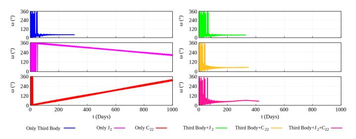
**Figure 10.** Diagram of  $\omega \times t$  showing different perturbative effects: considering only the perturbations by Uranus, only  $J_2$  from Titania, only  $C_{22}$  from Titania, Uranus  $+J_2$  from Titania, Uranus  $+C_{22}$  from Titania, and Uranus  $+J_2 + C_{22}$  from Titania. Initial values are  $a_i = 900$  km,  $e_i = 10^{-3}$ ,  $I_i = 80^\circ$ ,  $\omega_i = \Omega_i = 0^\circ$ .
