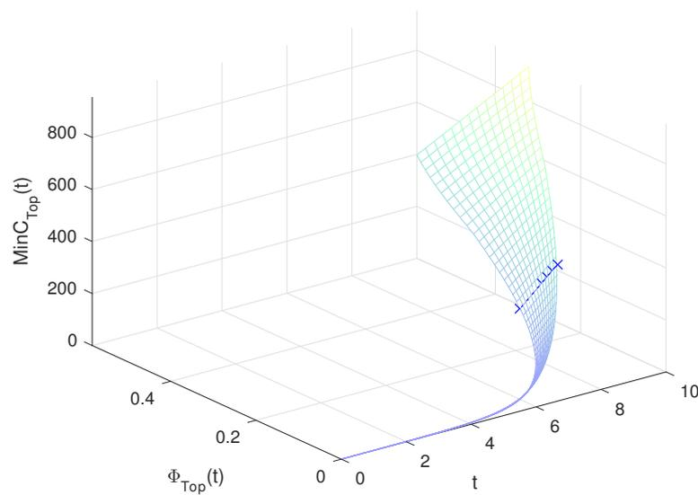
**Figure 3.** The relationship between maintenance time  $t$ ,  $\Phi_{Top}(t)$  and  $\text{Min } C_{Top}(t)$ .
