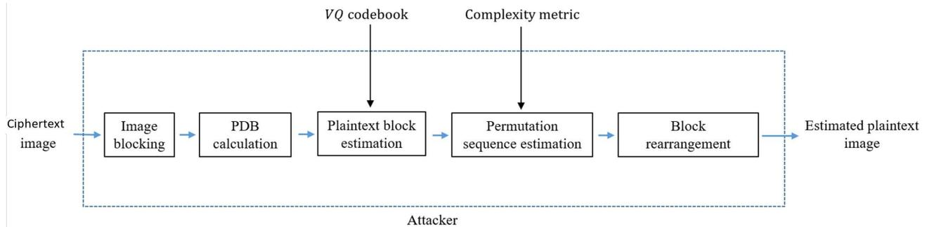
**Figure 2.** Flowchart of the proposed cryptanalysis method.
