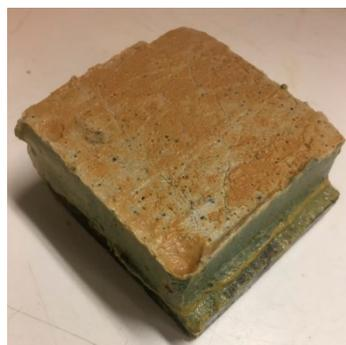
**Figure 8.** Specimens after the direct shear experiment (treated for 1 day; initial sulfate concentration of 25,000 mg/L; made with 0.3% fibers; normal stress of 50 kPa).
