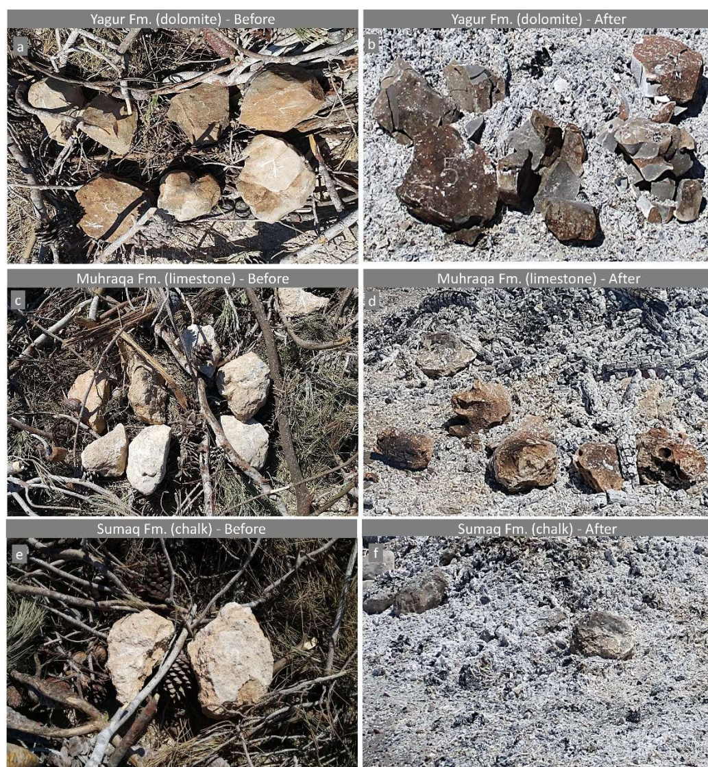
Figure 5. The boulder conditions “before and after” the open fire (where the temperature reached up to 880 °C); the dolomite boulders completely shattered, while limestone and chalk boulders cracked but only partially broke down.
