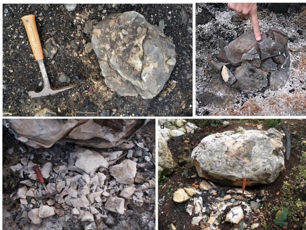
Figure 3. Boulder response to high temperatures: (a + b) moderate size boulders ( D < 0.5 m) completely disintegrate and shatter; (c + d) large boulders ( D > 0.5 ) usually exfoliate and partially shatter.
