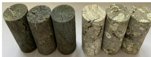
**Figure 3.** Specimens of triaxial compression test.
