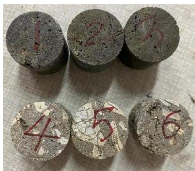
Figure 4. Specimens of Brazilian splitting test.
