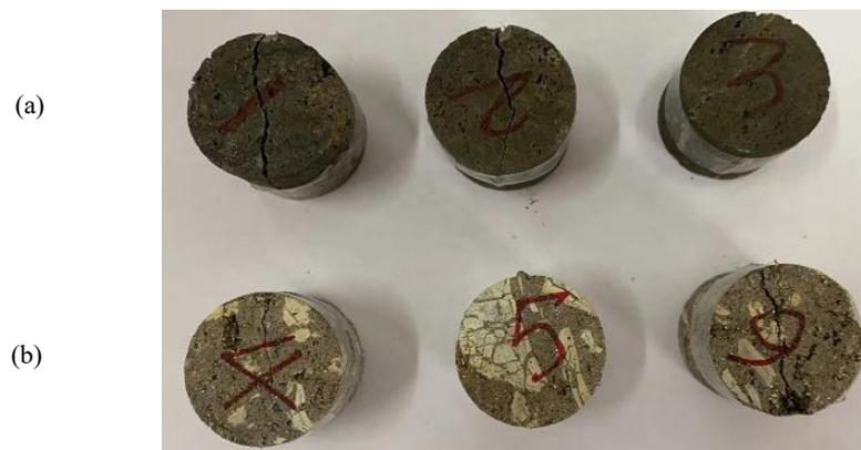
Figure 9. Brazilian splitting failure modes of two kinds of SMS samples. (a) Black; (b) White.
