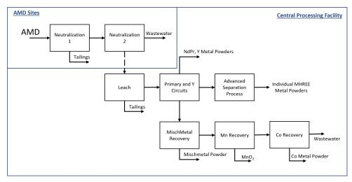
Figure 2. Proposed block flow diagram.
