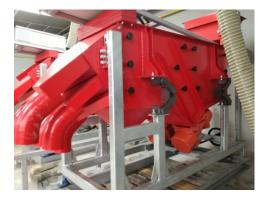
Figure 14. Six-product three-deck vibrating screen made by HTS Gliwice.
