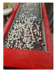
Figure 18. Screening process and production of regular particles on the three-deck vibrating screen.
