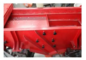
Figure 15. Three-deck vibrating screen with a separate receiving system for irregular particles.
