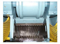
Figure 1. Jaw crusher to improve the grain shape.
