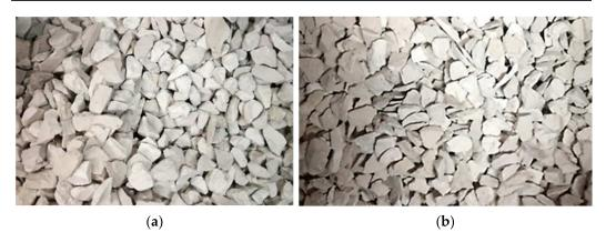
**Figure 20.** Limestone 12–14 mm, upper product, 99.3% regular particles, 10 mm× 60 mm screen (**a**), limestone 12–14 mm, lower product, 99.3% irregular particles, 7 mm× 60 mm screen (**b**).
