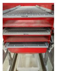
Figure 16. Screen decks and chutes after opening the screen head.
