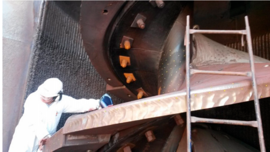
Figure 9. Scanning procedure to obtain a three-dimensional measurement of liner parts [30].
