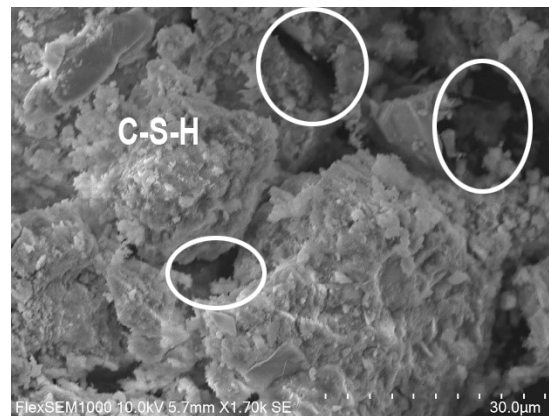
Figure 7. Concrete samples found in active sludge with an acidic pH following 345 d of the experiment.
