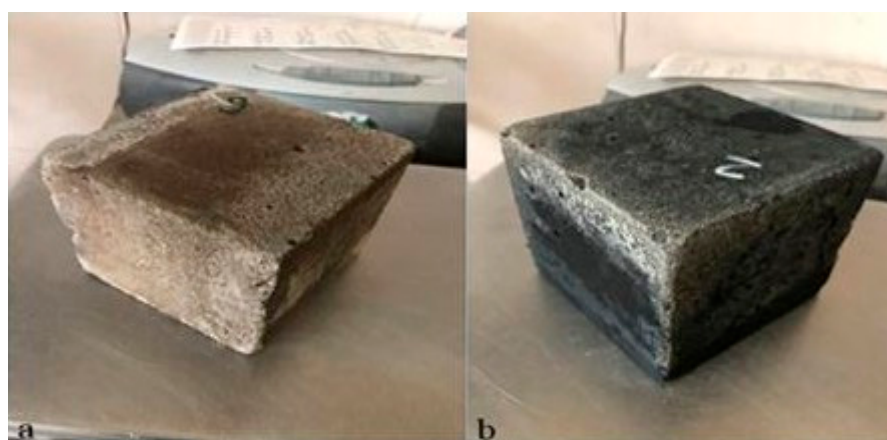
Figure 2. (a) Concrete samples found in post grit chamber sewage with an acidic pH; (b) concrete samples found in active sludge with an acidic pH.
