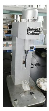
Figure 2. XFG-40 mL flotation machine with the flotation cell, dam board, and scraper.
