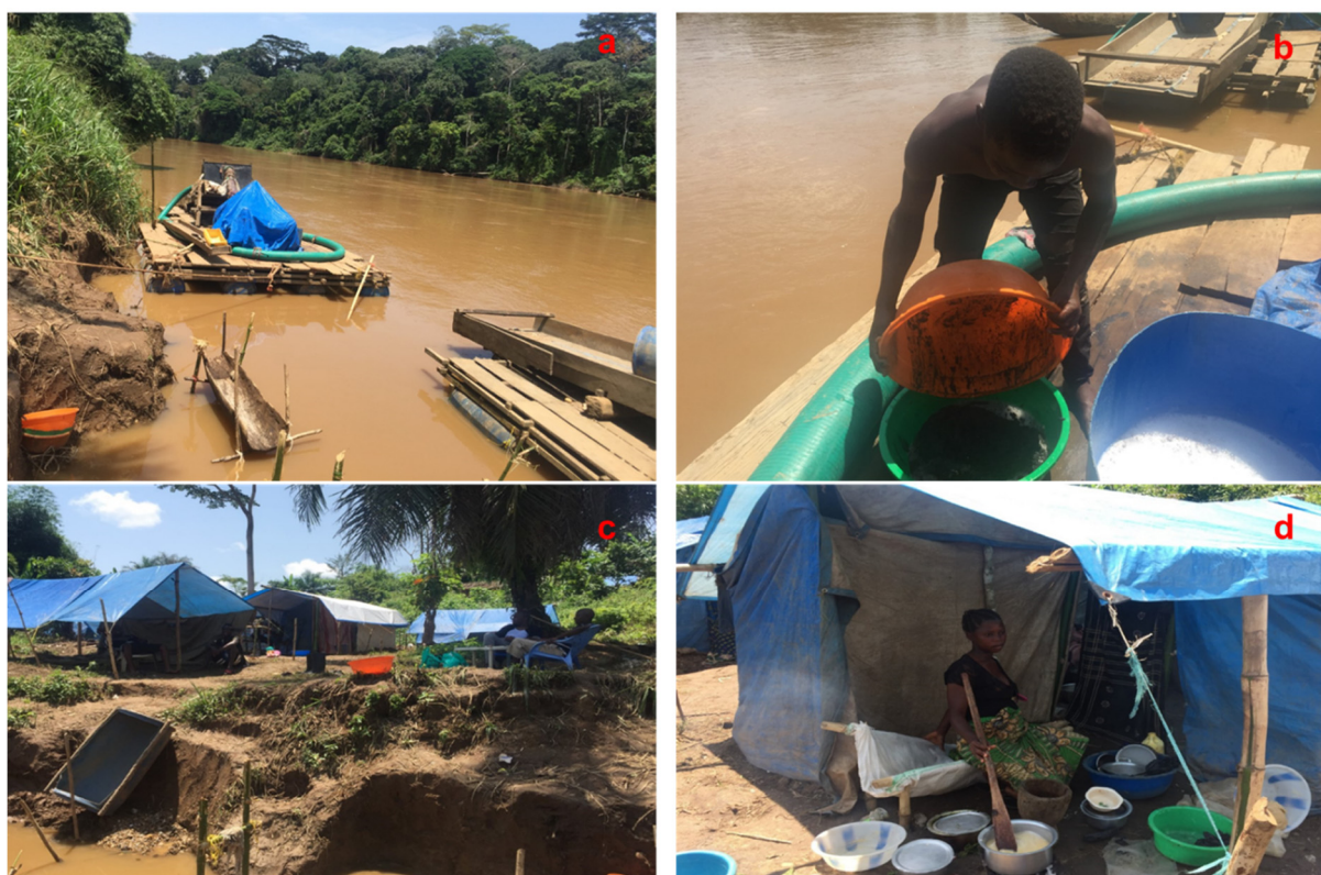
Figure 2. Artisanal and small-scale mining activities and miner's settlements along the Ulindi River. (a): dredge used for gold mining, (b): addition of Hg to form the amalgam with gold, (c): miner dwellings, (d): food cooking on the river bank (Photos by E. Atibu).
