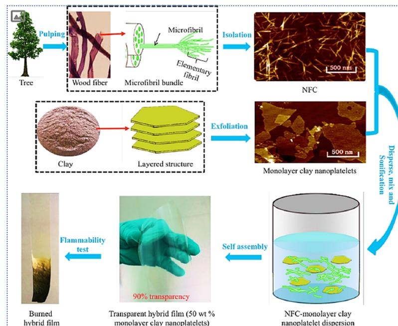
**Figure 4.** Schematic of transparent nanofibrillated cellulose (NFC) monolayer/nanoclay nanoplatelet-based hybrid films with self-extinguishing behavior (90% transparency at 600 nm). One-dimensional
