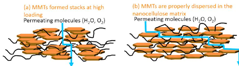
**Figure 8.** Mechanism of MMT stacking and arrangement of stacks in nanocellulose network. (a) MMT stack formation at high loading level which decrease the tortuous path; (b) MMT stacks broken down using high-pressure homogenization of nanocellulose/MMT suspension which increase the tortuous path [183]. MMT = montmorillonite. Reproduced with permission from Elsevier.
