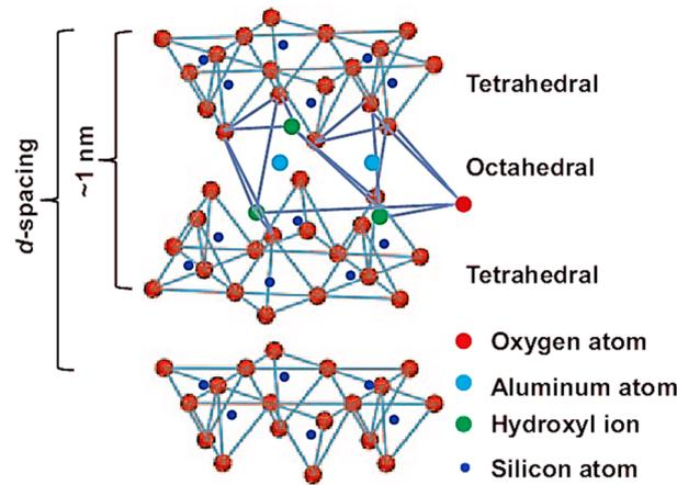
Figure 1. Structure of nanoclay (montmorillonite) [44]. Reproduced with permission from Springer.
