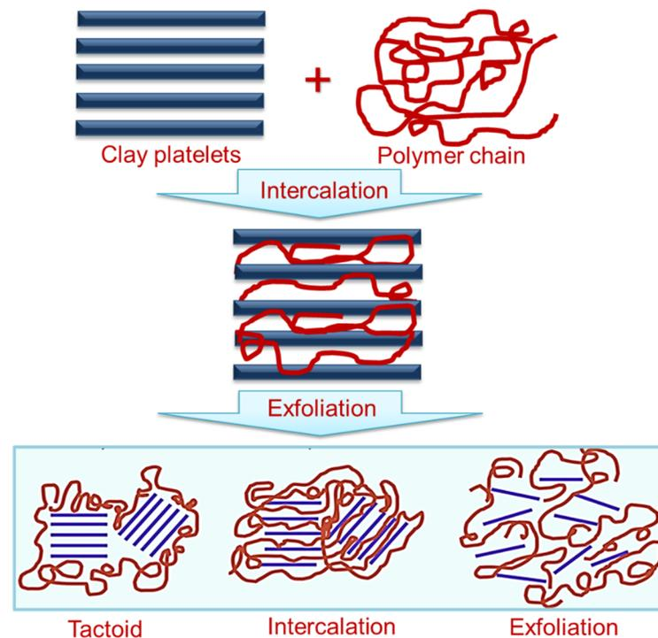
**Figure 3.** Formation of polymer/layered silicate nanostructure via intercalation and exfoliation.
