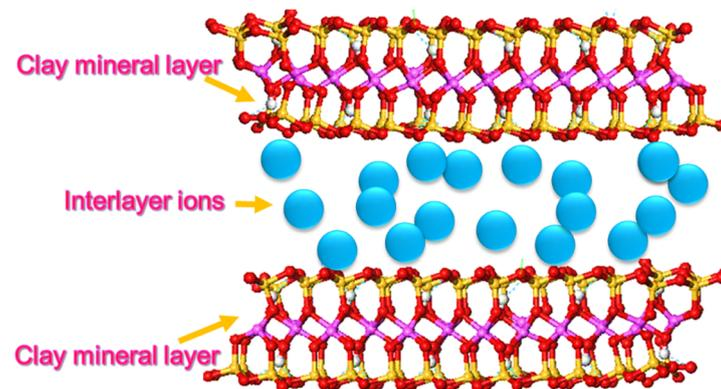
Figure 2. Entrapment of ions in layered nanosilicate nanostructure.
