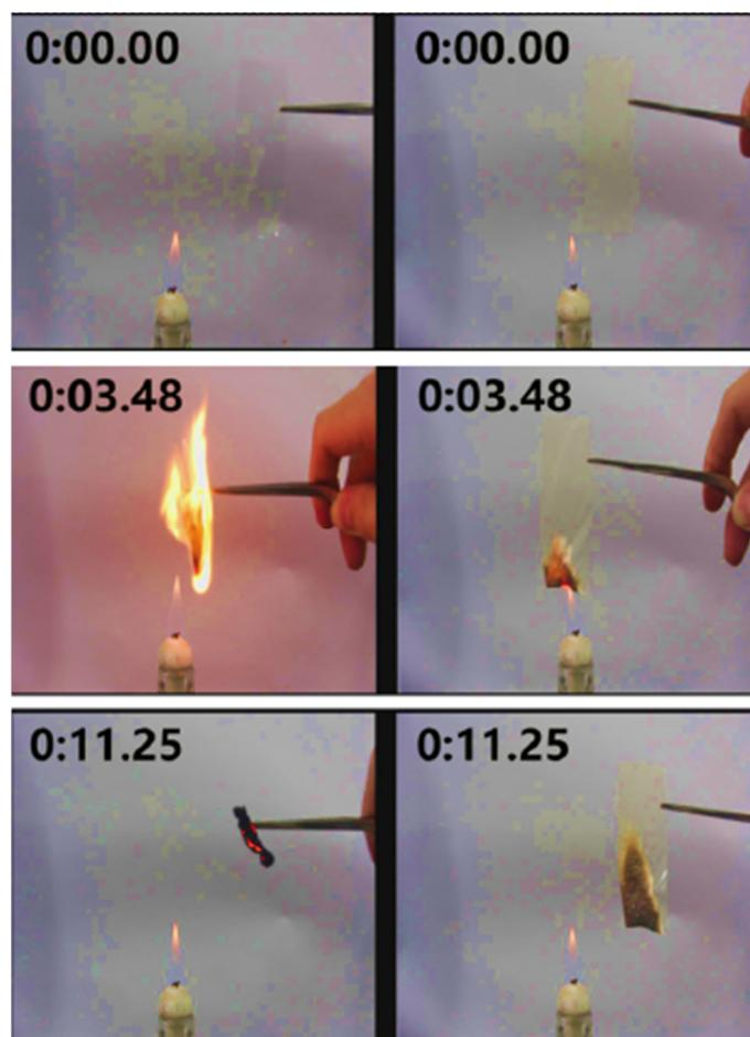
**Figure 5.** Time-lapse flammability of (left) pure nanofibrillated cellulose film and (right) transparent hybrid film with 50 wt.% monolayer clay nanoplatelet, respectively [113]. Reproduced with permission from ACS.
