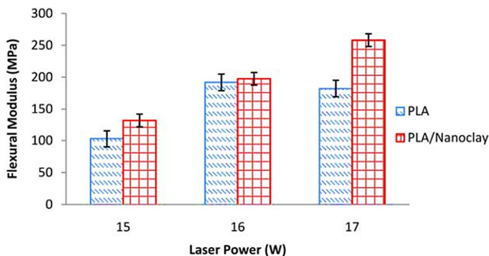
**Figure 6.** Variation in flexural modulus vs, laser power for poly(lactic acid) and poly(lactic acid)/montmorillonite nanoclay nanocomposite (powder bed temperature 60 °C) [138]. Reproduced with permission from Wiley.
