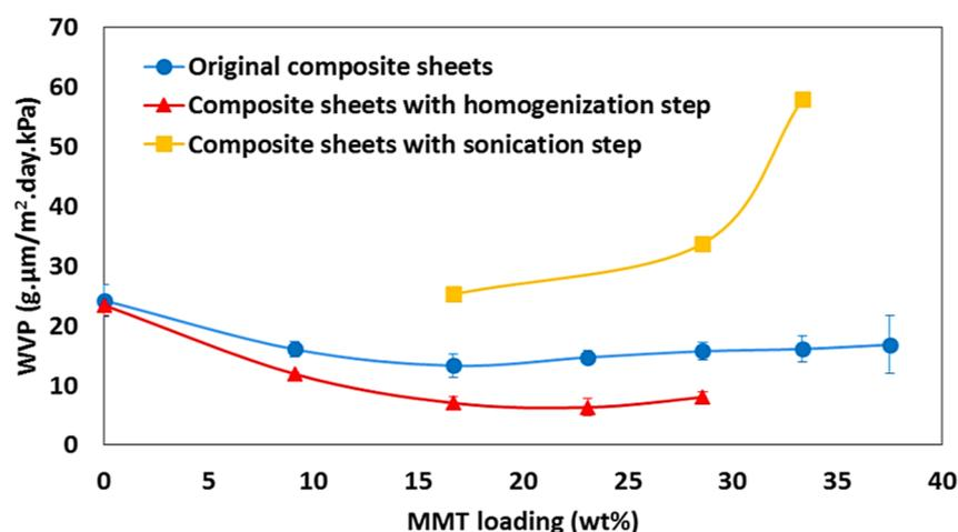
**Figure 9.** WVP of nanocellulose/MMT nanocomposites. The pristine nanocomposite sheets; nanocomposite sheets with high pressure homogenization step, and sonication step [183]. WVP = water vapor permeability; MMT = montmorillonite. Reproduced with permission from Elsevier.
